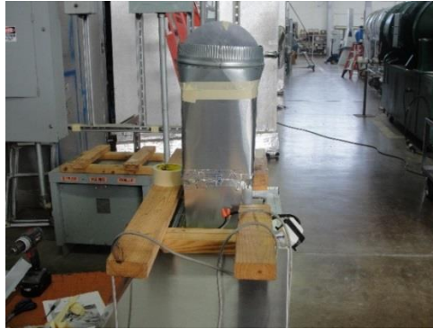
Figure 23: Duct Discharge Extension Modification (Code: DDE)
