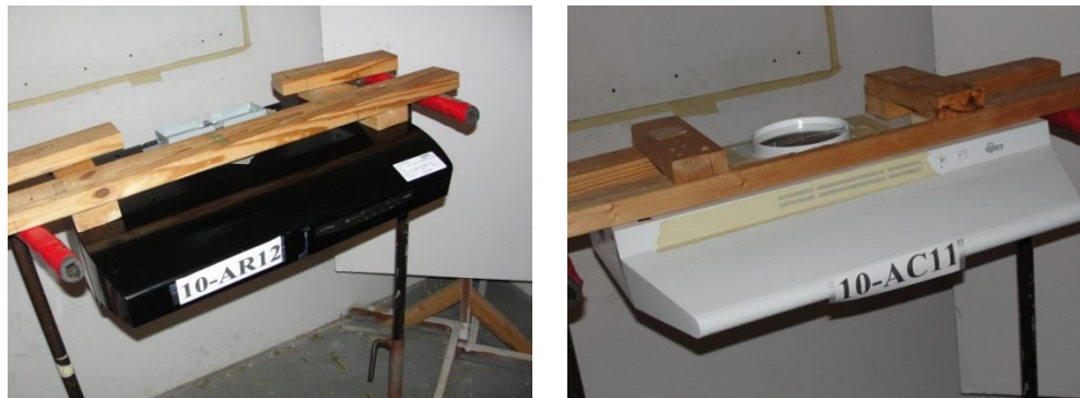
Figure 11: Axial Fan Kitchen Range Hoods Used for Testing
