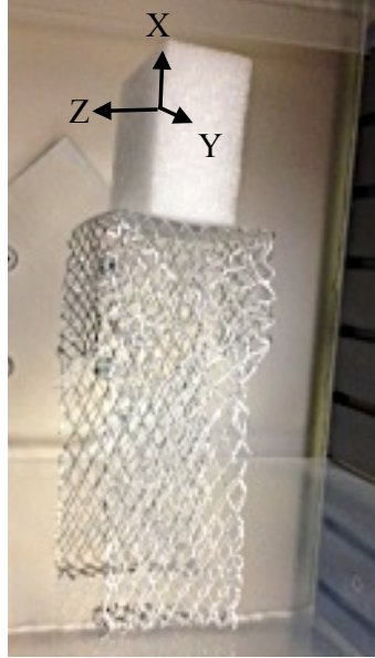
Figure A-7: Fifth stage, S5, evaluated using Process 12 to improve reticulation homogeneity throughout ultra-low density shape memory polymer foam block sample. S5 consisted of a 50.8 x 50.8 x 127 mm (L x W x H) aluminum mesh stage, allowing the sample to be elevated 127 mm above the glass shelf in the reaction chamber. S5 was utilized while orienting the foam with such that the foaming direction was perpendicular to the electrode.
