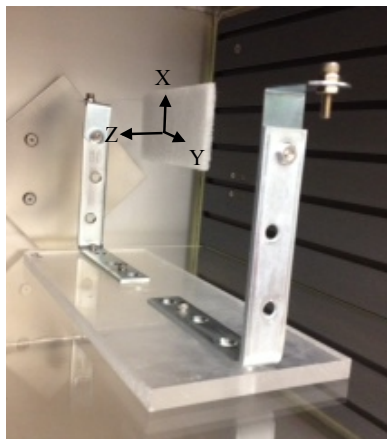
Figure A-8: First sample stage for plasma reticulating ultra-low density shape memory polymer foam sheet samples, S6. The sample stage was made of two stainless steel L-brackets screwed into a PMMA base, and a 0.2 mm diameter nitinol wire suspended between the L-brackets. The sheet samples were threaded onto the wire along the 101.6 mm edge, allowing the sample to be elevated 114.3 mm above the glass shelf. The samples were oriented such that the foaming direction was perpendicular to the electrode.
