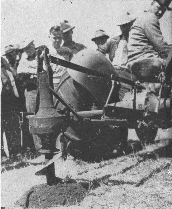
This view of the digger shows how it looks from the tractor driver's seat. Only one operator is needed. The device is easy to attach to a Ford tractor and can be lowered or raised readily.
