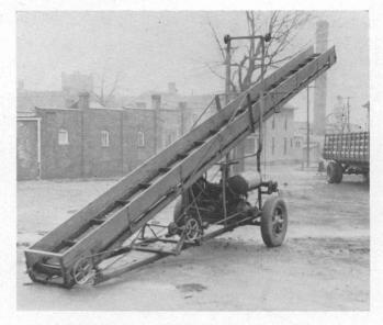
Baled hay elevator for lifting bales into the barn. (Courtesy of University of Illinois)
