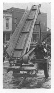
Baled hay elevator which also may be used for ear corn. Standard manufactured steel link chains are generally used. Steel attachment links and sprockets are also manufactured parts. Flights may be made of angle iron or wood.
