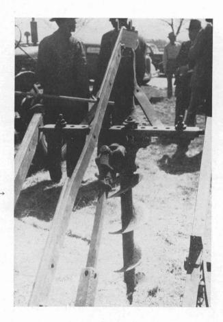
The rear end of a Model A Ford provides a basis for this digger. The top axle is cut off flush with the housing and welded to the housing to keep it from turning. A pipe is fitted over the remaining axle to which a gin auger is welded. Cutting blades are welded on at the tip to make the digger take the
