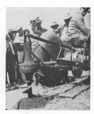
This post-hole digger was developed by Jack Woodson, foreman of the Circle Bar Ranch in Lubbock County. It digs holes 30 inches deep at the rate of two per minute. This machine was built entirely of scrapped materials. The only cost was for welding.
