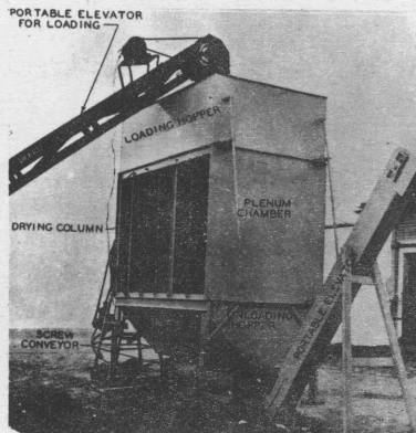
Fig. 5. A batch-type dryer developed by the Texas Agricultural Experiment Station with major parts labeled. Units operating on the same principle are available commercially. Heated air is required and close supervision is necessary but drying capacity is relatively high.
