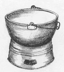
The fire is made in the tub, and the wash kettle set in the opening. A grate could be placed over the opening for other uses.
