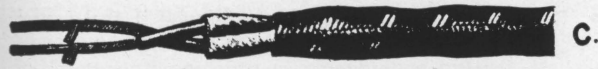
a. light usage cord b. hard usage cord c. heating appliance cord
