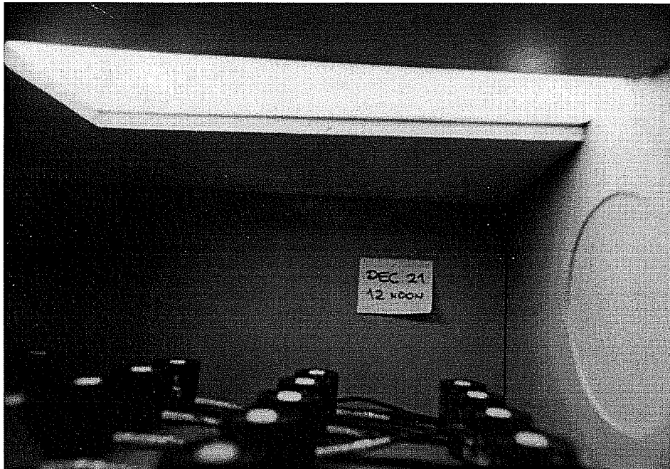
Figure 17. Photograph of one Light Pipe C at December 21, 12:00 PM, 34°N.
