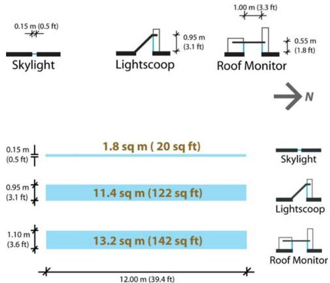
Fig. 1: Cross sections and glazing area comparison of single unit prototypes
