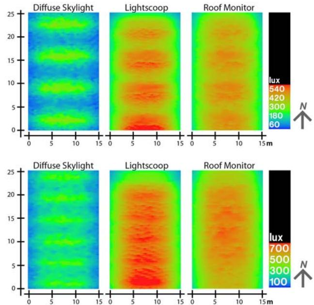
Fig. 7: Illuminance distribution over floor plans rendered with RADIANCE of SHR 1.5:1 (top) and SHR 1:1 (bottom), overcast sky
