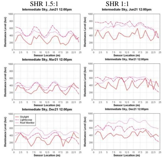
Fig. 6: Comparison of illuminance levels of SHR 1.5:1 and 1:1; under CIE intermediate skies, 12:00pm
