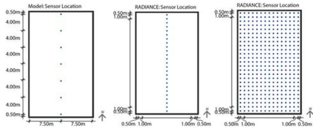
Fig. 5: Plan view of sensor location in scale model (left), RADIANCE model for DF (center), and uniformity analysis (right)
