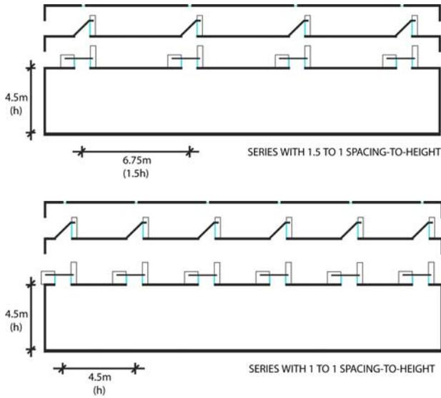
Fig. 2: Cross sections of the prototypes with SHR 1.5:1 (top) and SHR 1:1 (bottom)
