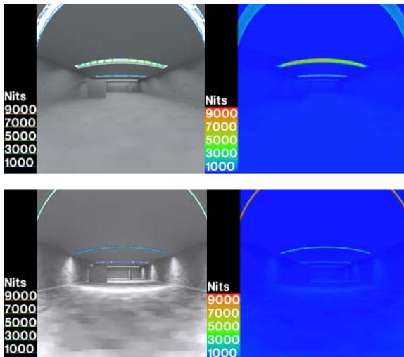
Fig. 8: RADIANCE images of interior space with roof monitor (top) and skylights (bottom) with SHR 1.5:1, June 21 at 12:00pm, CIE clear sky
