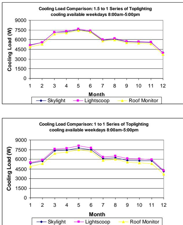
Fig. 3: Comparison of cooling loads, SHR 1.5:1 (top) and 1:1 (bottom)
