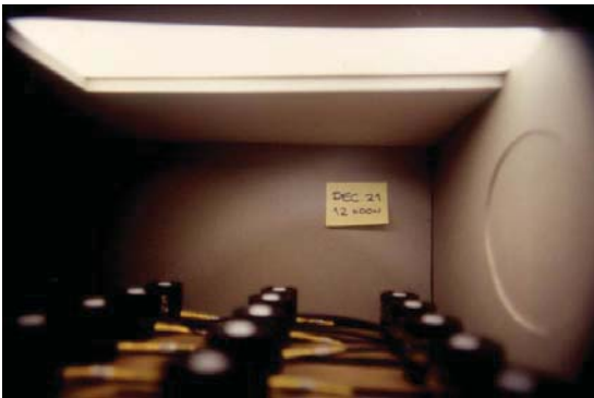
Fig. 1. Interior views of scale models with light pipe: without sidelight window (left), and with window (right).
