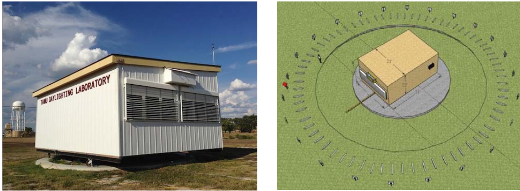
Fig. 5. Exterior view of room (left), and sketch of room rotation every 15° (right).
