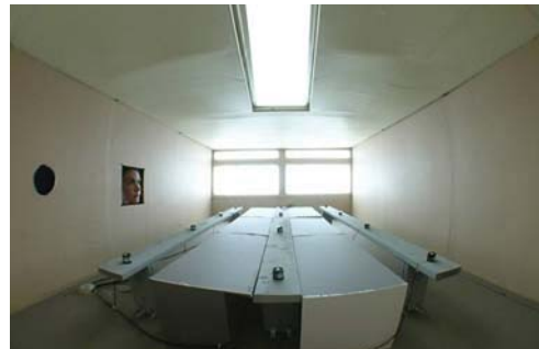
Fig. 2. Two large scale models: test and reference models (left), and interior view of test model showing light pipe (right).
