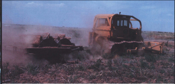
Figure 8. Roller chopping reduces noxious brush and increases forage production through its influence on the water availability.
