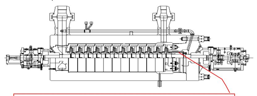
Straight drum on the right is used for balancing axial thrust with return of balancing line to the pump suction nozzle
