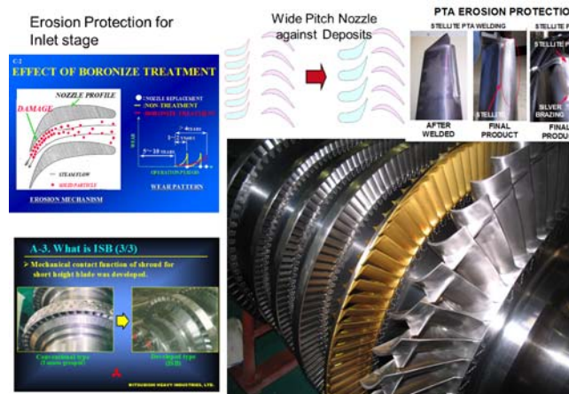
Figure.37 Surface Treatment Application for Steam Turbines
