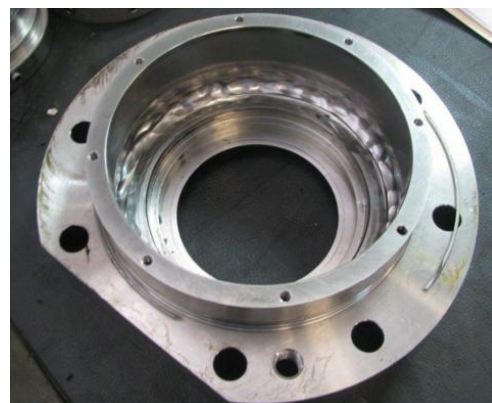
Figure 2: Mechanical seal faces damaged by dry running and sand erosion
