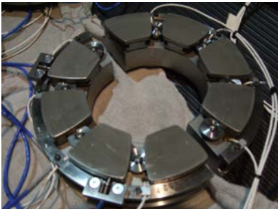
Figure 18. Equipped thrust device
