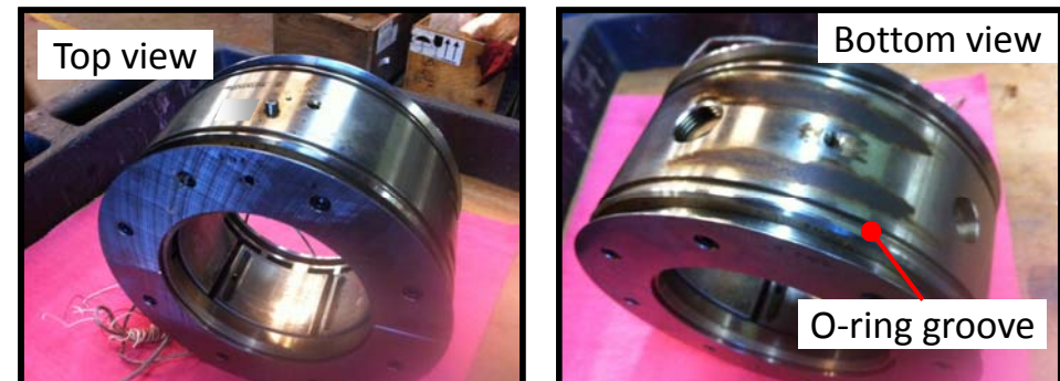
Fretting damage on bearing OD
