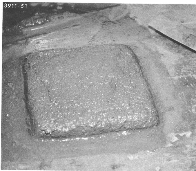
(a) Wet trowelled preform
