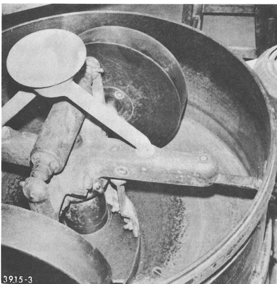
(c) Roll grinding apparatus (fibrillator)
