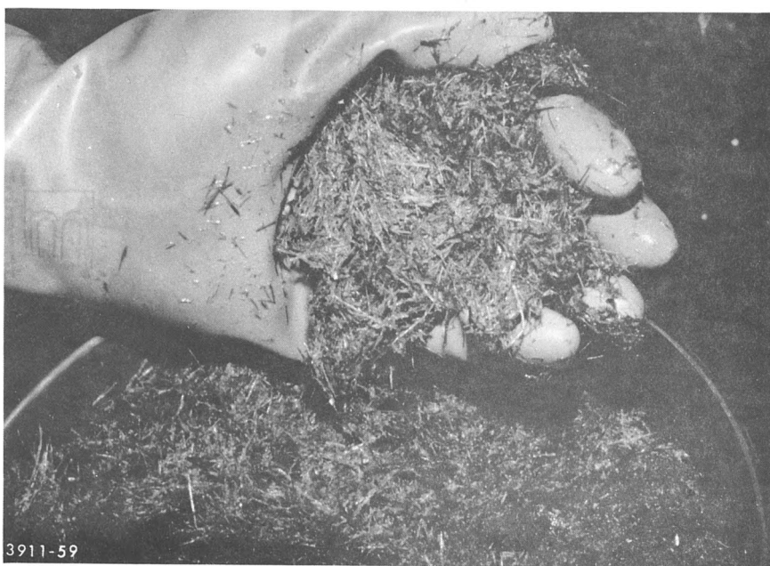
(b) Fibers with pith washed out
