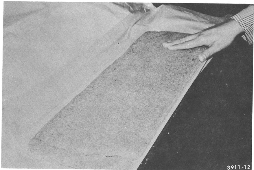
(a) Oriented preformed bagasse mat
