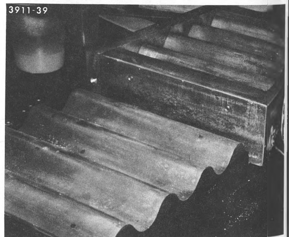
(c) corrugated electrically heated mold
