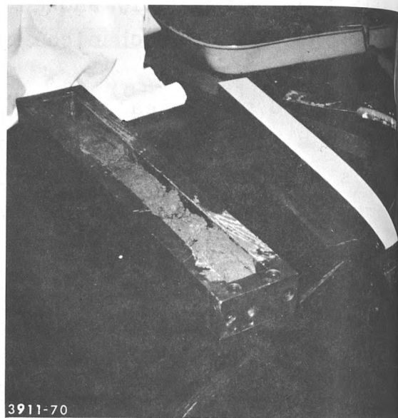
(b) Wet compound in compressed mold
