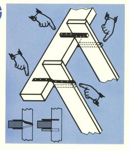
Fasten your roof joists to both sides of the rafters to prevent twisting.
