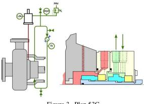
There are some significant advantages to this approach. The pressurization source for the system is the process fluid in the pump itself. There is no need for an external pressure source. The barrier fluid is automatically pressurized as the pump is commissioned. This removes this step from the normal
