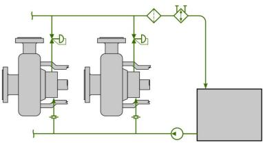
Note: Instrumentation and redundancies not shown for clarity. Figure 7 Plan 54 Multiple-seal Support System
