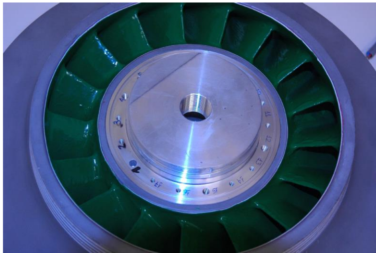
Fig. 3: Coated impeller before erosion test
