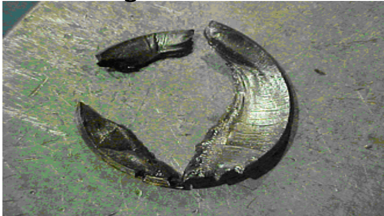
Fragments of the piston rod thread region
