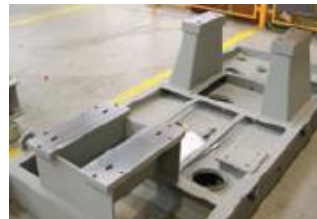
Figure 6: Sloped deck plate mounted between the side rails deck/top-plate and extending only under pump and coupling
