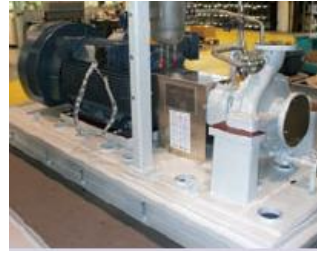
Figure 4: Flat deck type with a mounted sloped gutter drain and extending beneath the pump and driver
