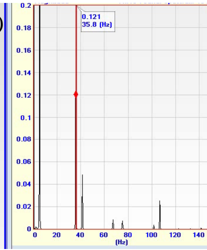
Fig 10. Natural Frequencies and Mode Shapes – based on FFT of 4 seconds following Fig 7 Impact
