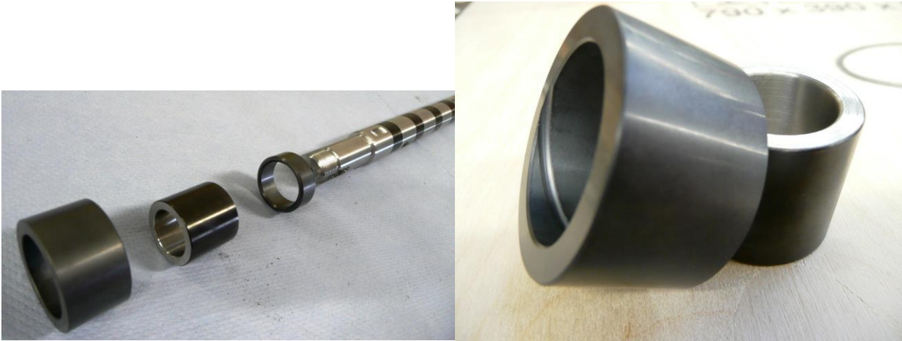
Figure 23: Silicon carbide bearing bushings w/ hard faced shaft
