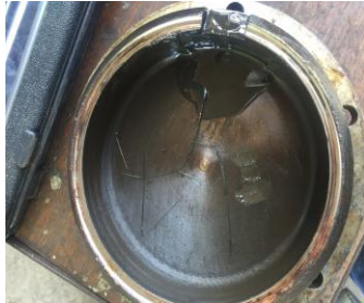
Wear in thrust bearings end cover by about 3 mm
