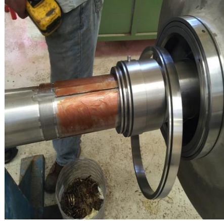
Rotor assembly and balancing , check casing wear rings and throat bushings clearances measuring
