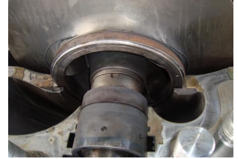
DE throat bushing stuck on shaft
