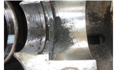
Deformation in casing housing for DE throat bushing first stage Casing Wear ring inside
