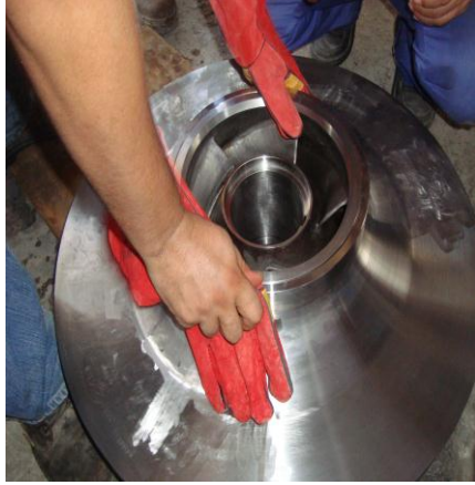
Rotor assembly and balancing , check casing wear rings and throat bushings clearances measuring
