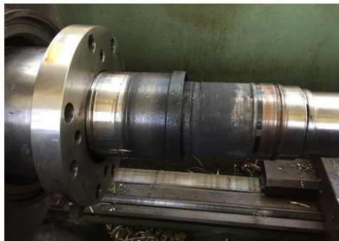
DE Throat Bushing stuck with M/C rotary sleeve
