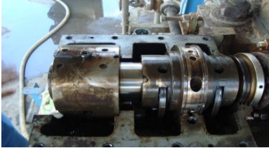
Inner side casing wear ring of first stage impeller
