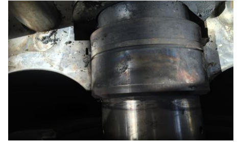
Deformation in casing housing for DE throat bushing first stage Casing Wear ring inside
