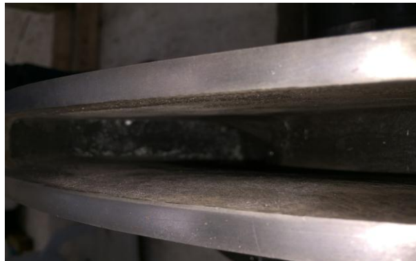
Potassium Carbonate solidification inside impeller
