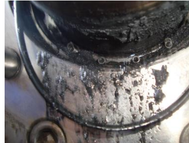
Damage of DE Mechanical seal
