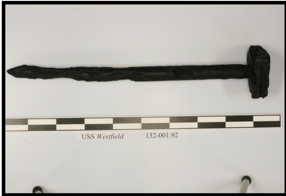
Figure 90. Type 2 massive bolt fastener for cylinder base/bed frame timbers (Artifact 132-001.92; scale dm.).
