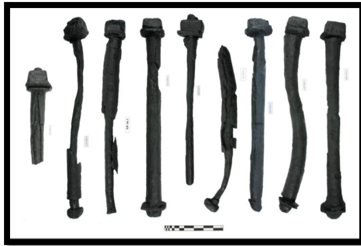
Figure 111. Large staybolts from upper steam drum (scale inches).
