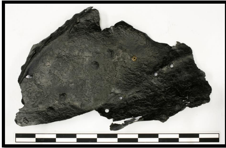
Figure 154. Plate from the upper fire box water jacket (Artifact 124-032; scale dm.).
