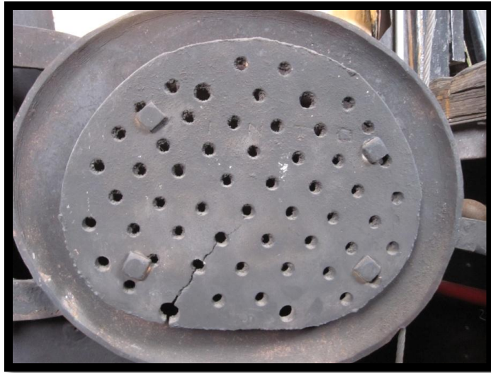
Figure 148. Baffle plate from the steamboat Moyie (Image courtesy of SS Moyie National Historic Site of Canada).
