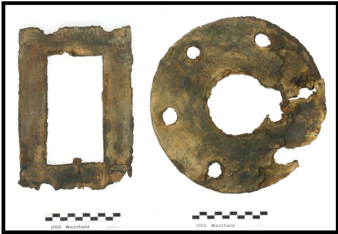
Figure 84. Examples of intact composite fabric gaskets from the valve assembly (Artifacts 132-017.6 and 132-017.8; scale cm.).
