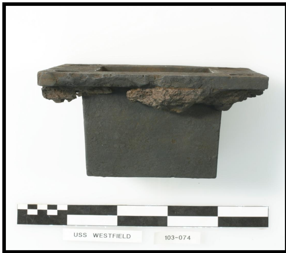
Figure 40. Stanchion socket from USS Westfield (Artifact 103-074; scale cm.).
