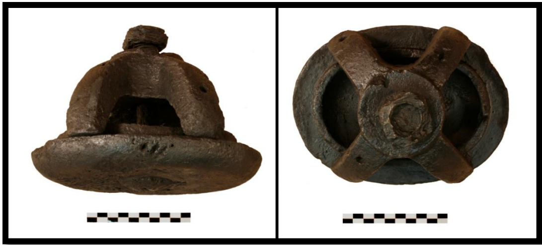
Figure 124. Medium sized hand hole cleaning cover (Artifact 118-178; scale cm.).
