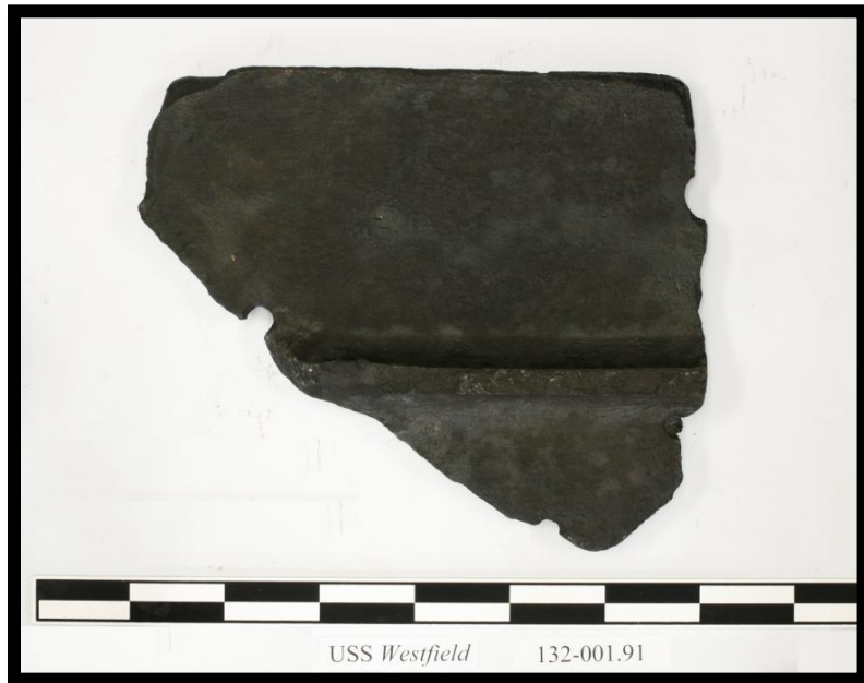
Figure 77: Fragment of port side base plate (Artifact 132-001.91; scale dm.).
