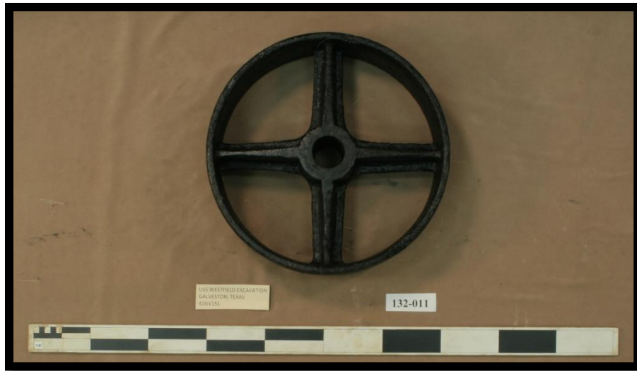
Figure 184. Cast iron wheel from a donkey engine (Artifact 132-011; scale cm./dm.).
