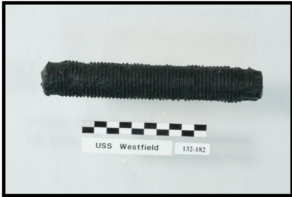
Figure 175. Threaded staybolt with hammered ends (Artifact 132-182; scale cm.).
