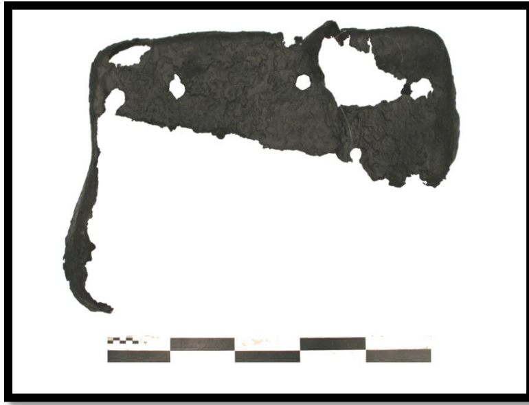
Figure 153. Flue door from Westfield's boiler (Artifact 109-127; scale cm./dm.).
