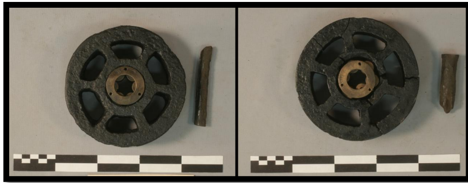
Figure 188. Cast iron sheaves with cupreous bearings (Artifacts 120-308 and 128-016).
