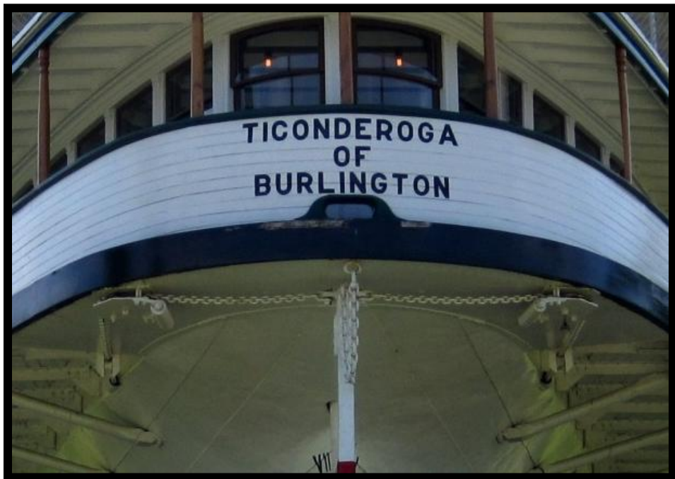
Figure 56. Rudder chains on the steamboat Ticonderoga (Image courtesy of the Shelburne Museum, Shelburne, Vermont).
