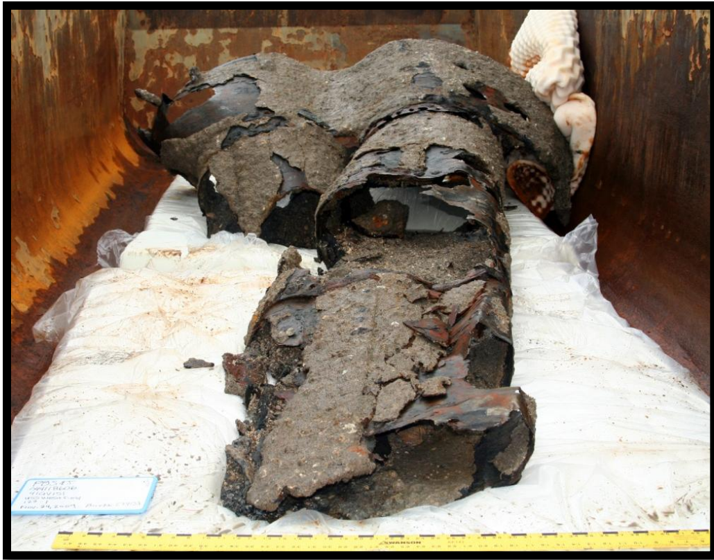
Figure 169. Westfield's boiler flues, upside down in a storage container (Artifact 122-001; scale inches).
