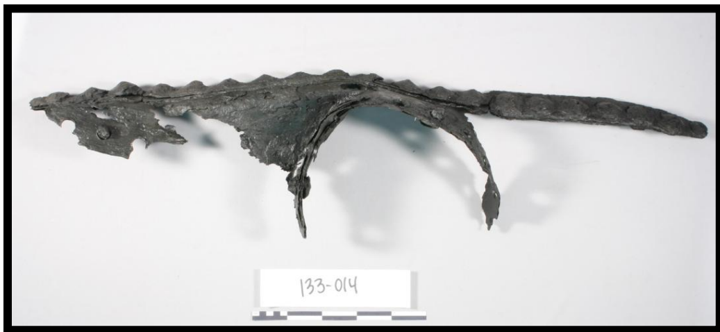
Figure 170. Plating designed to hold a smaller round flue (Artifact 133-014; scale cm./dm.).
