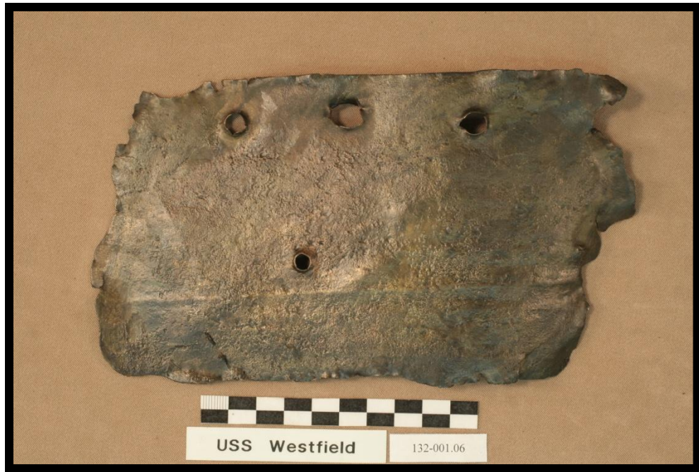
Figure 57. Copper hull sheathing (Artifact 132-001.06; scale cm.).
