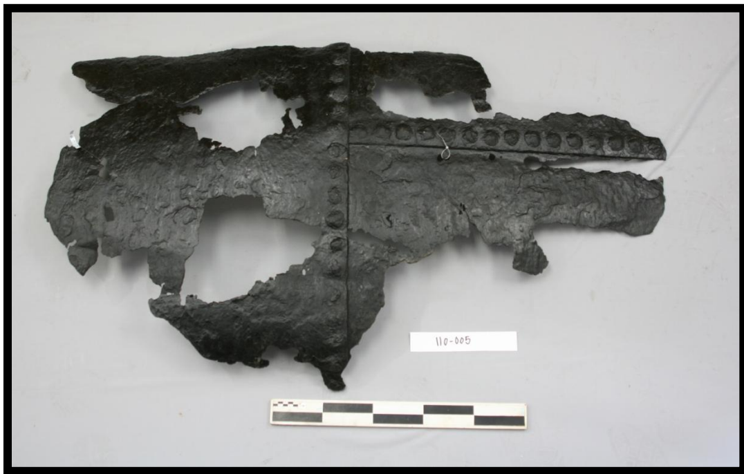
Figure 156. Large section of plating from the outer boiler barrel (Artifact 110-005; scale cm./dm.).
