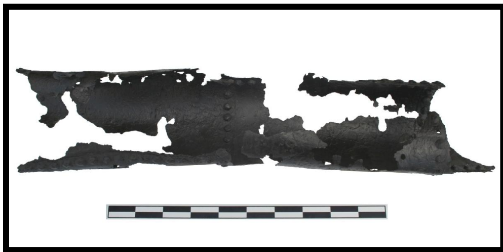
Figure 172. Smaller upper side flue on Westfield (Artifact 121-010; scale dm.).
