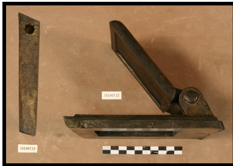
Figure 85. Cupreous valve and wedge from the valve assembly (Artifacts 132-017.12 and 132-017.13).
