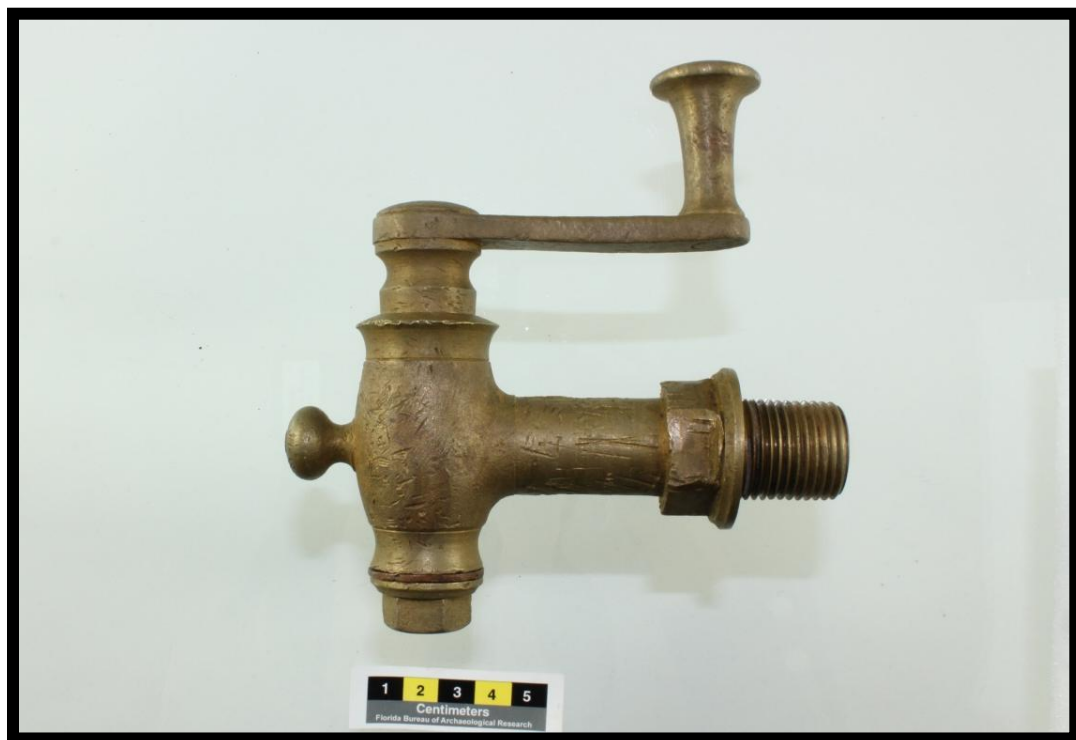
Figure 64. Cupreous water cock gauge from USS Maple Leaf (Image courtesy of Florida Bureau of Archaeological Research).
