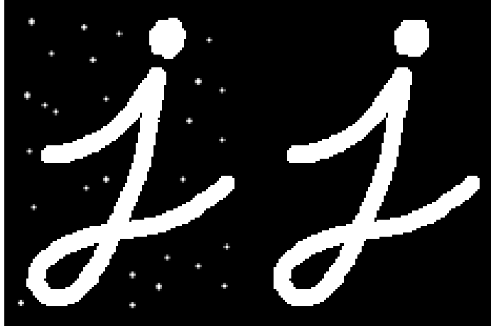
Figure 1.12: Input image (left) prior to a morphological opening operation. Output image (right) maintains the figure of interest's shape while removing speckle noise. Holes within the figure would also be removed from the image by this procedure. (OpenCV-Python Documentation, 2014)
