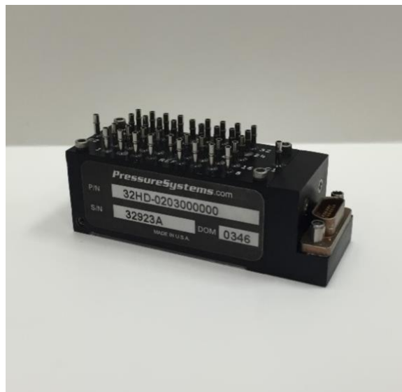
Figure 4.6: Pressure scanner with tubing.
