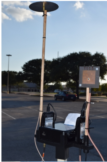
Figure 5.1: Monitoring device setup with Intel™ NUC and custom antenna designs.
