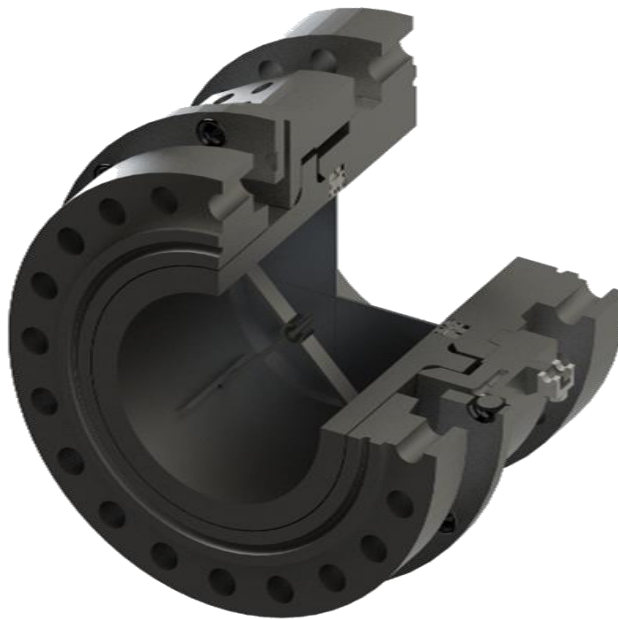
Figure 35. Hydraulic pin holder placed in the breech head with four mounting arms and a blank body that can receive multiple pin configurations.
