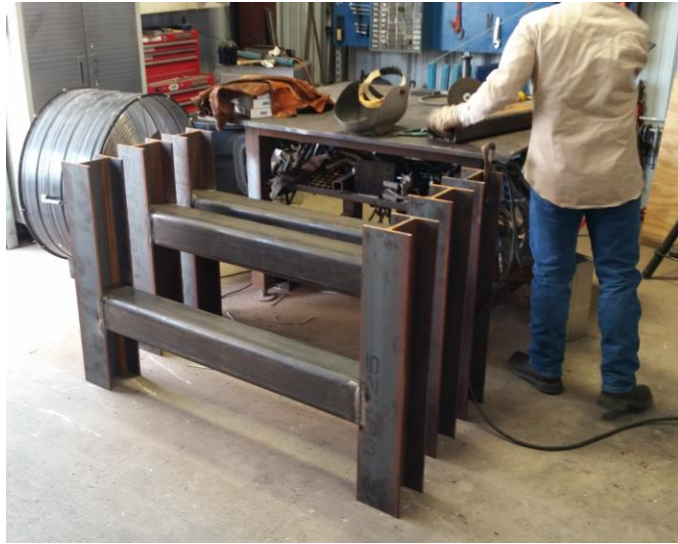
Figure 81. H-shaped central bodies welded together being prepared for the 2-inch thick main plate.
