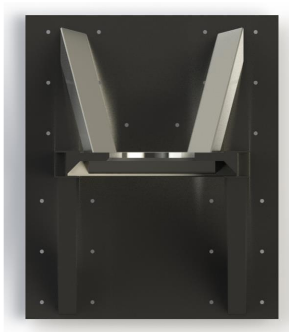
Figure 73. Overhead view of the secondary stands with emphasis on the movement of the back I-beams to connect with the H-beam instead of the 2-inch thick plate.
