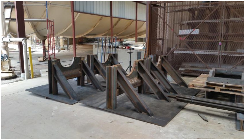
Figure 105. Four of the five stands tacked together without the 6-inch square tube bracings.
