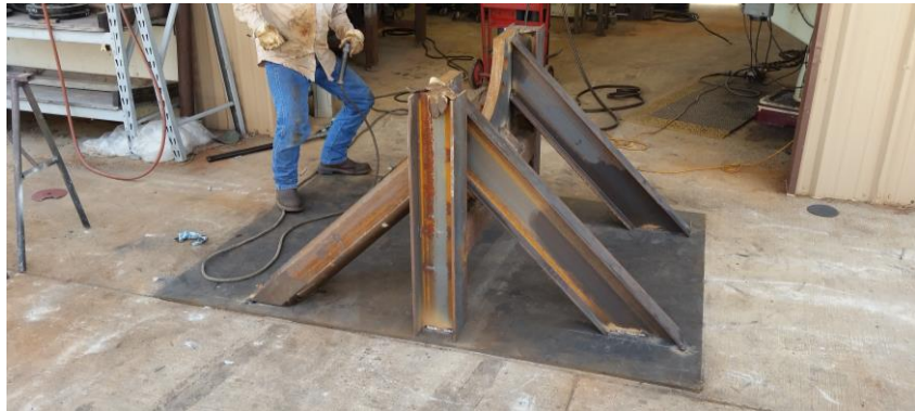
Figure 84. Driver-side primary stand fully tacked into place.
