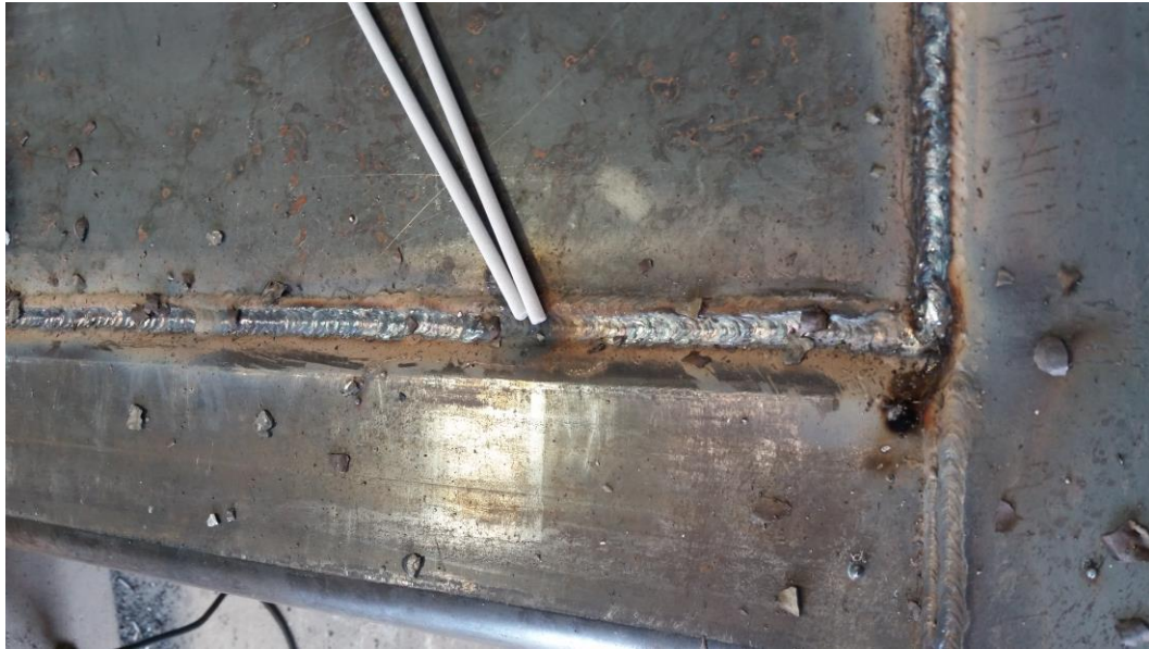
Figure 80. Example picture of the welds performed on the 2-inch thick plate to the H-shaped central body.
