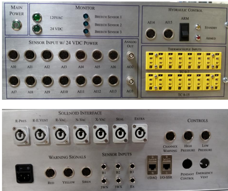
Figure 93. (Top) Front panel and (bottom) back panel of the control and instrumentation hardware interface electronics housing.
