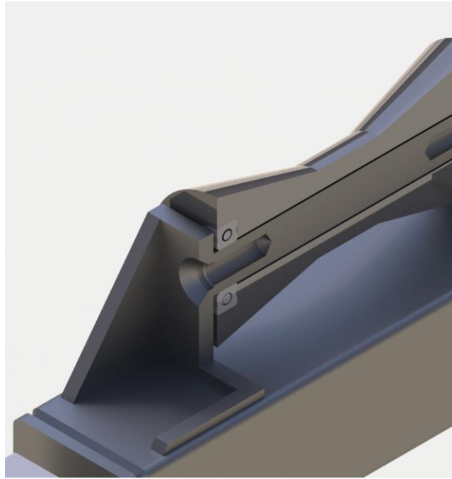
Figure 79. Cross sectional cut of the roller detailing the position of the ball bearings and threads in the axle.
