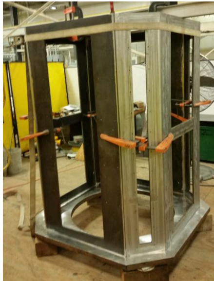
Figure 60. Test section pieced together and clamped just before welding.
