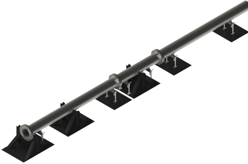
Figure 16. Computer aided design model for accelerator pipe as it appears with a 900# flange on the driven side of the segment, structural stands, and roller supports.
