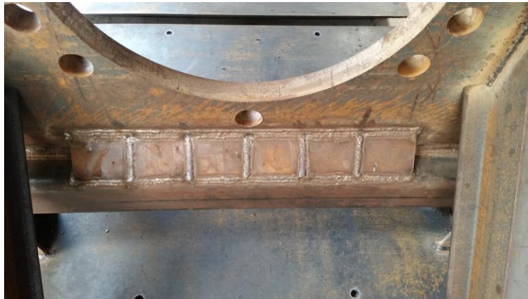
Figure 82. Close up of the main gusset divided into six manufacturable pieces and welded to the stand.
