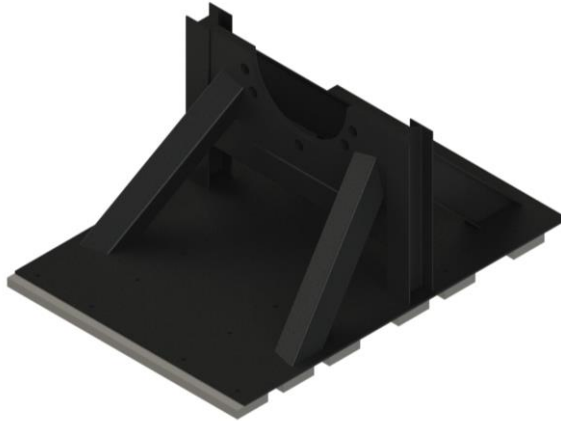
Figure 67. Representation of how the stands may be shimmed to achieve proper height.
