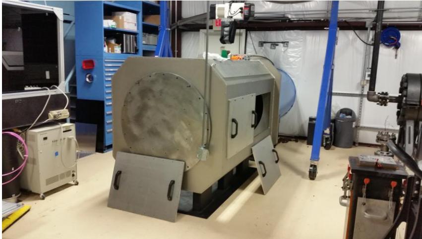
Figure 104. Back assembly with test section and tailpipe running through the wall of the NAL with blind adapter plate for eventual hydrostatic pressure testing.
