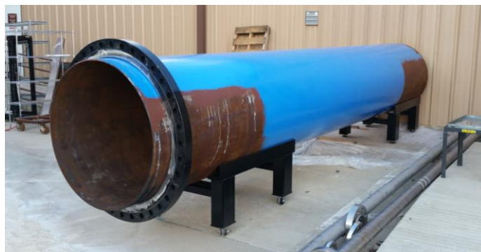
Figure 61. Tailpipe immediately before the 42” 150# slip-on flange was welded to the end of the pipe.
