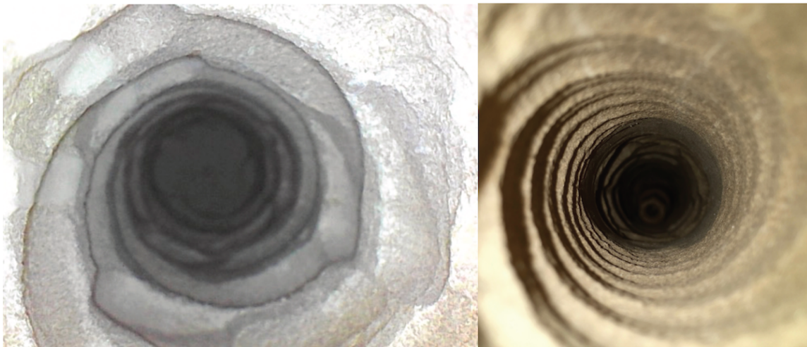
Figure 5.10: Borehole patterns caused by excessive bit whirl
