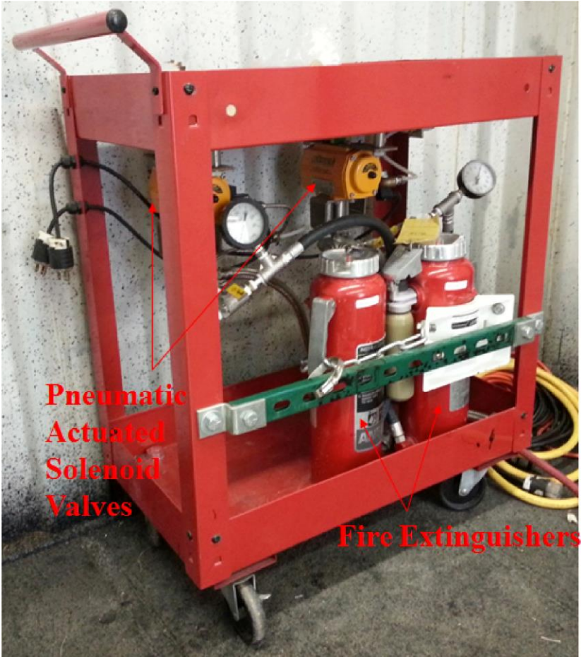
Figure 7: Fire extinguisher cart
