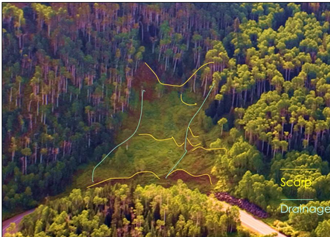
Figure 5. Aerial image of the Donald Duck Landslide Complex. Landslide scarps are drawn as well as modern surface drainage. Aug. 2011.
