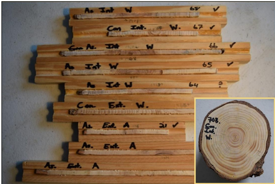
Figure 13. Cores and cookie. Examples of aspen and conifer in core. The conifer cookie demonstrates the complexity of movement at the junction of the three slides. Personal photos, March, 2015.
