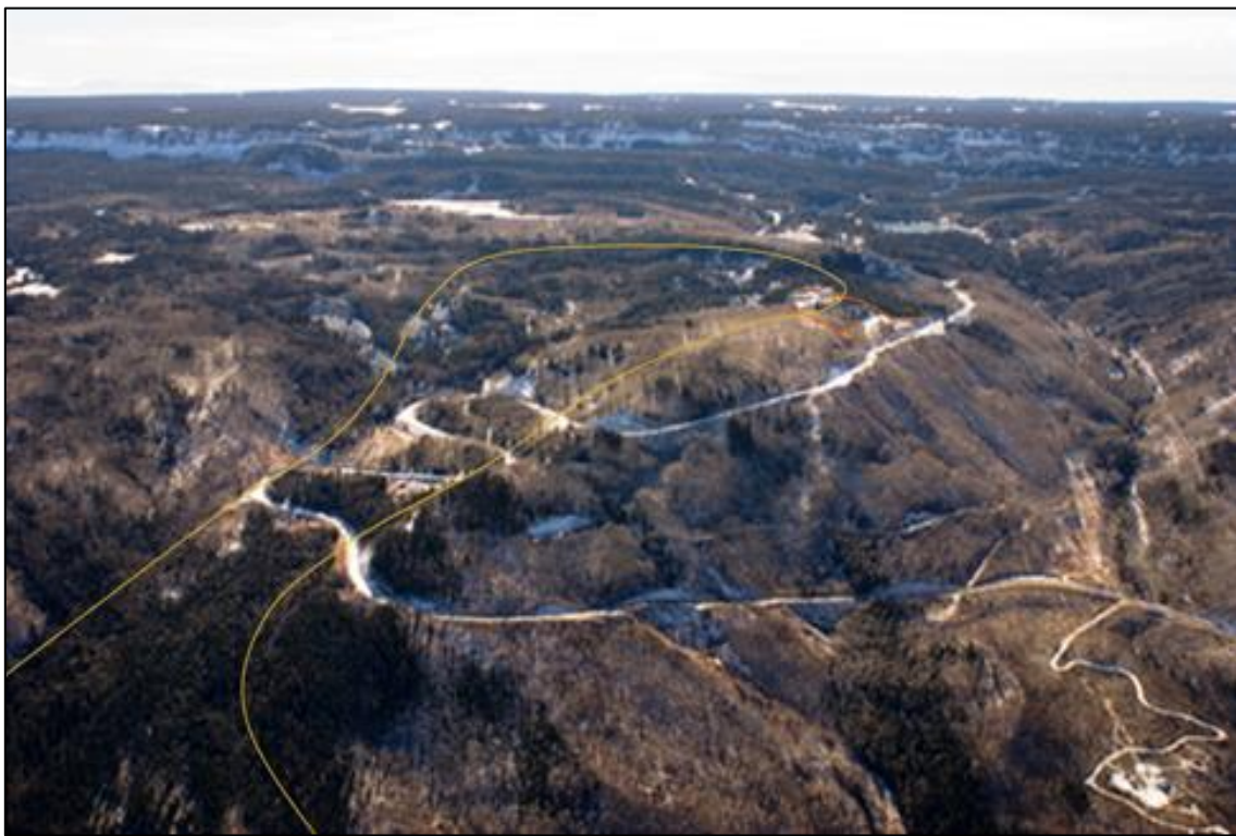
Figure 7. Outline of the ancient landslide. The gold line outlines the ancient landslide. The landslide underlies the entire valley occupied by the SH 65 switchbacks. Google Earth, Jan. 2014.
