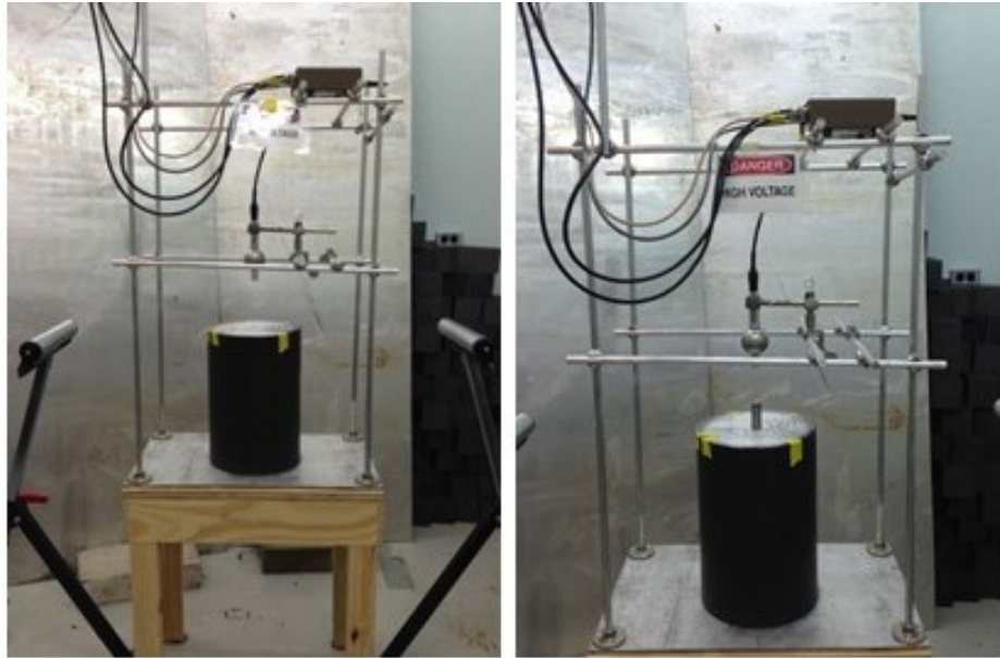
Figure 2.4: Experimental setup with the source in the HDPE shield (left) and in the minimalist configuration (right).
