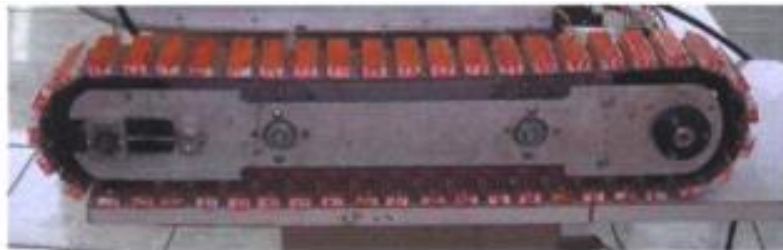
Figure 3-2: Magnetic track developed for the robot SIRUS [20].
