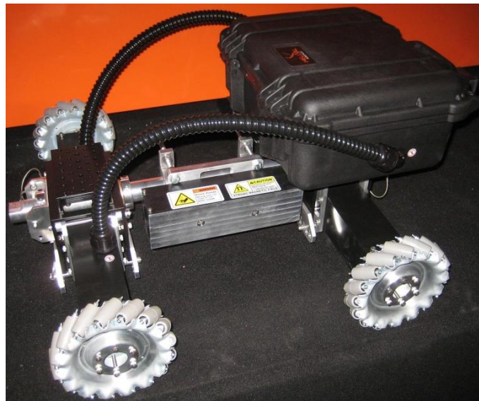
Figure 3-5: FerroTanker-20 robot featuring a large magnet under its body [23].
