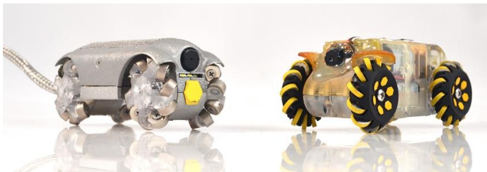
Figure 3-3: Pipe inspection robot developed by Honeybee Robotics [21].
