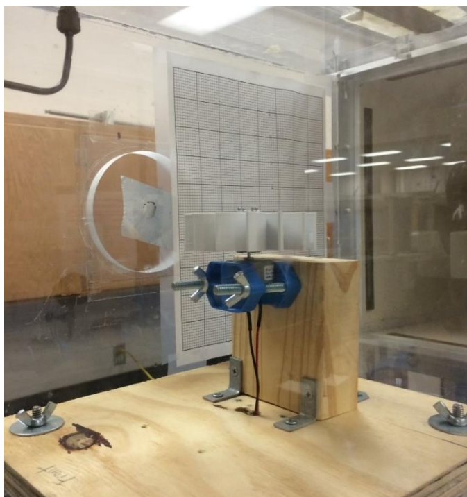
Figure 4-6: Test stand used to conduct experiments for turbine selection.
