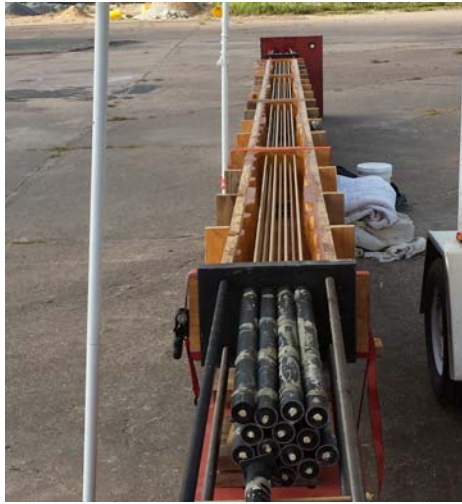
Figure 33: Fully stressed AFRP bars just prior to concrete pour
