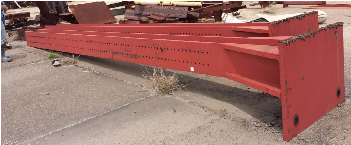
Figure 68: I-Beams to be used for prestressing frame
