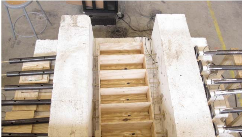
Figure 12: Creep-rupture test set-up (Medina 2011)
