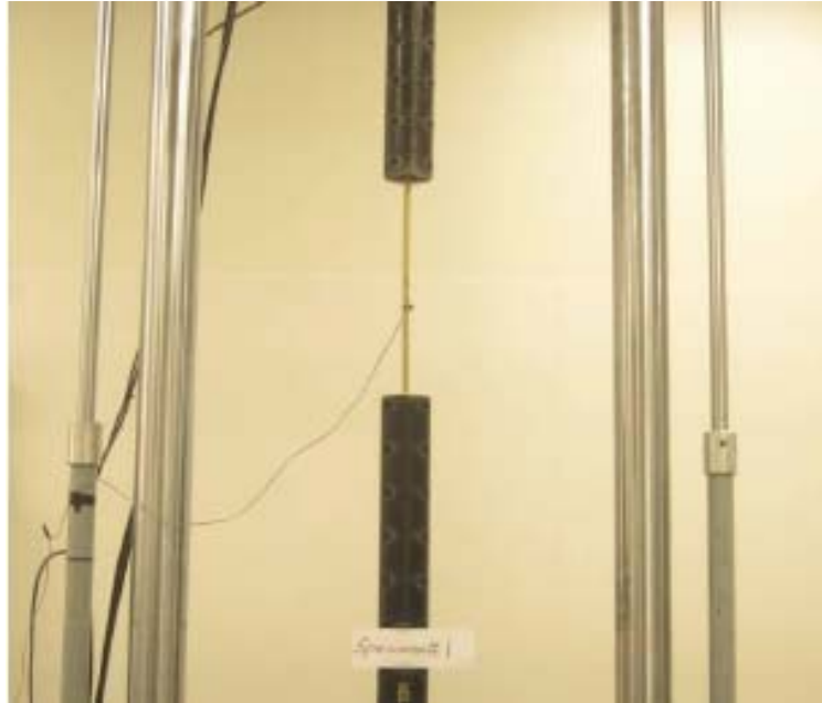
Figure 10: Tensile test of AFRP bars (Medina 2012)
