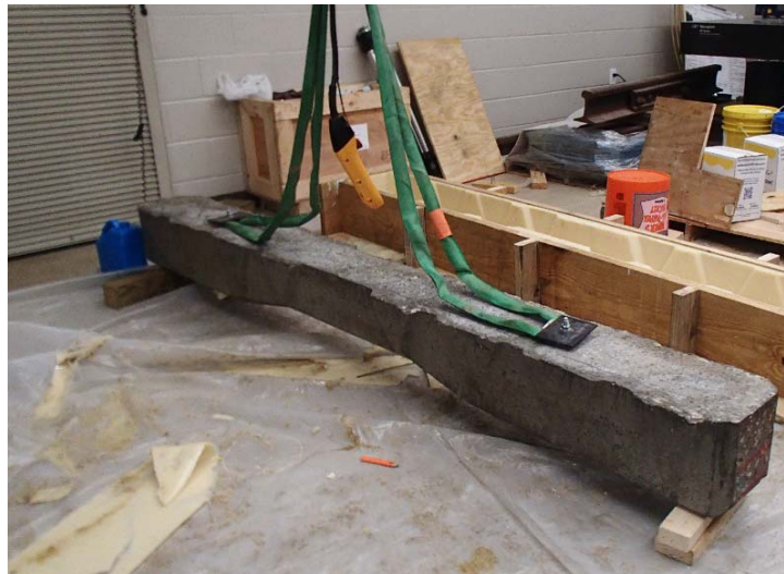
Figure 28: Original tie with anchor bolts and straps used for lifting in and out of box
