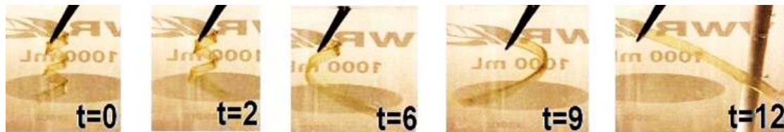
Figure 7 – Images showing shape recovery from a secondary helical geometry to a primary flat geometry in 12 s at 37°C for the DCHMDI-0.00 SMP
