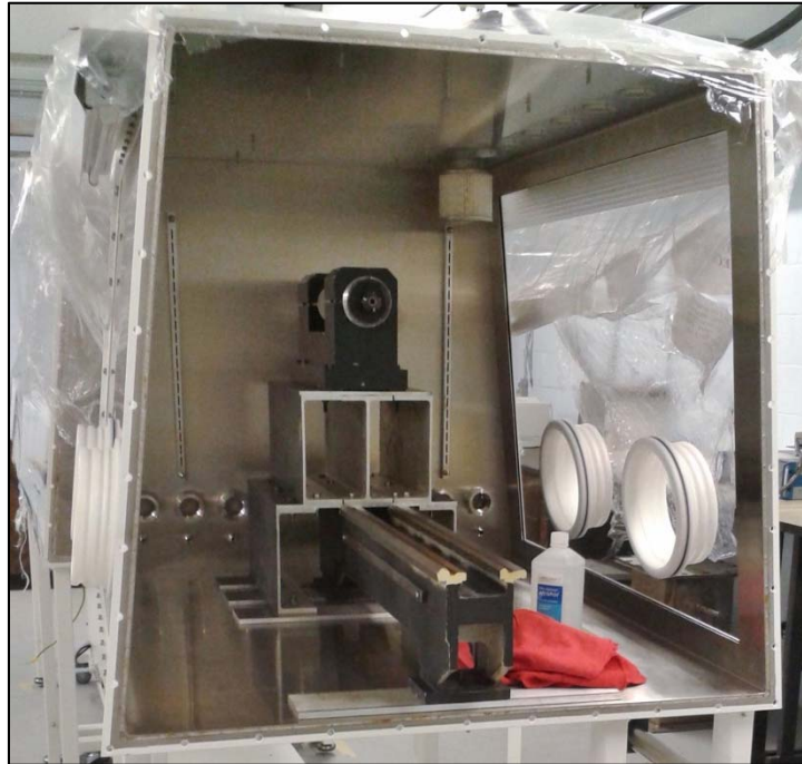
Figure 3-21: Pieces of the larger rotating electrode system components inserted into the glovebox before closure.
