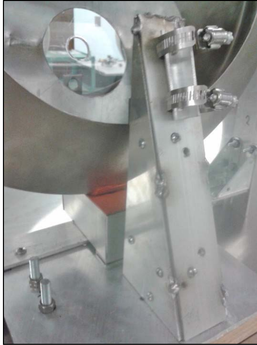
Figure 3-37: Torch holder tack-welded together
