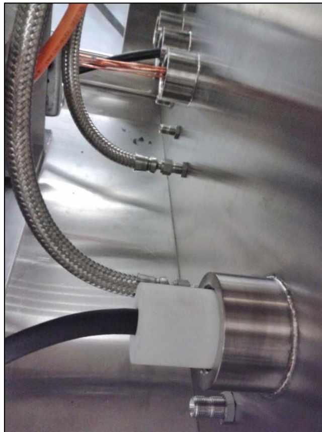
Figure 3-36: Interior view of all five glovebox feedthroughs
