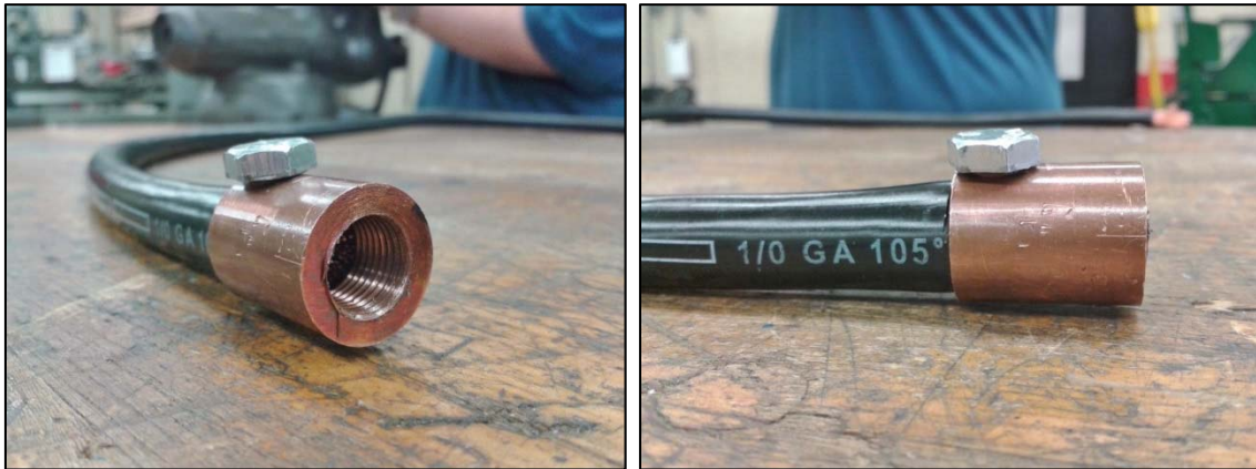
Figure 3-34: EG-500 copper adapter with set screw
