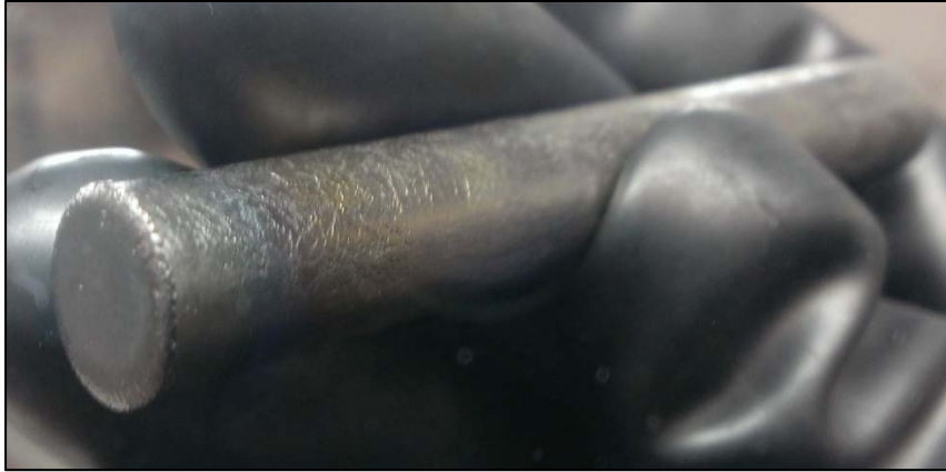
Figure 4-30: The Melt tip of a uranium rod after atomization
