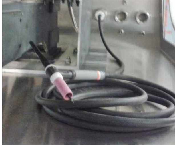
Figure 3-30: TIG welder torch connected to EGT-750 gland seal via Ultra-Flex tubing
