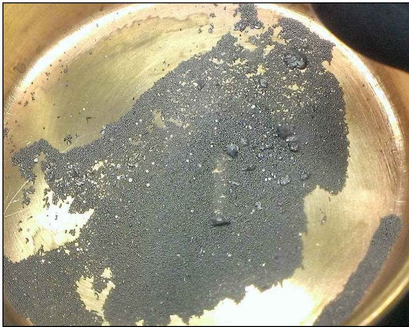
Figure 4-29: Uranium powder before characterization
