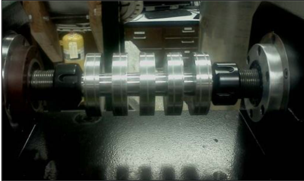
Figure 3-3: Photograph of the slip ring mounted between the two spindles [1]
