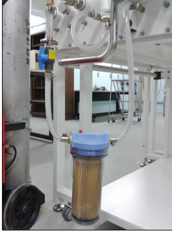
Figure 3-23: Water filter for the motorized spindle cooling water
