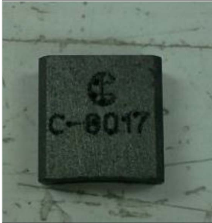
Figure 3-10: A single LFC544 electro graphitic brush fabricated by Mersen [1]
