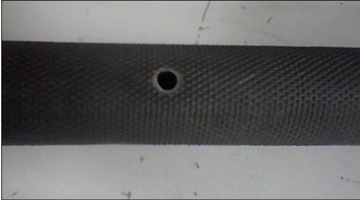
Figure 4-1: Hole burned through the torch handle cover as a result of arcing
