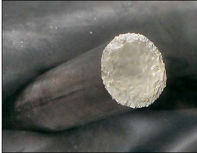
Figure 4-36: The melt tip of the 18,000 RPM U-10Zr rod after atomization
