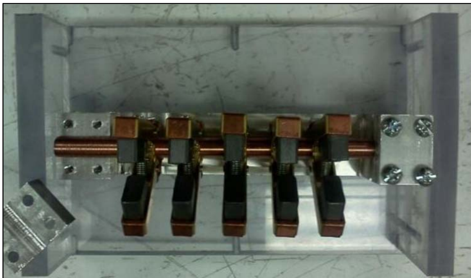
Figure 3-12: The five brush holders mounted to the 1cm diameter copper rod [1]
