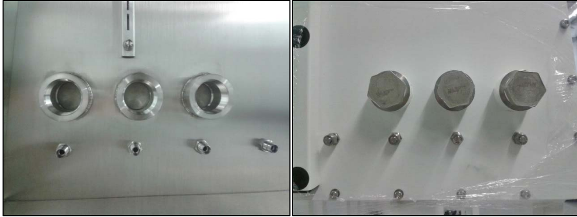
Figure 3-25: Inside (left) and outside (right) views of the two types of feedthroughs into the glovebox
