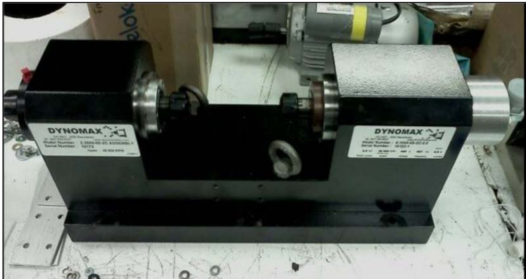
Figure 3-4: Photograph of the Dynomax Spindle Holder with spindles installed [1]
