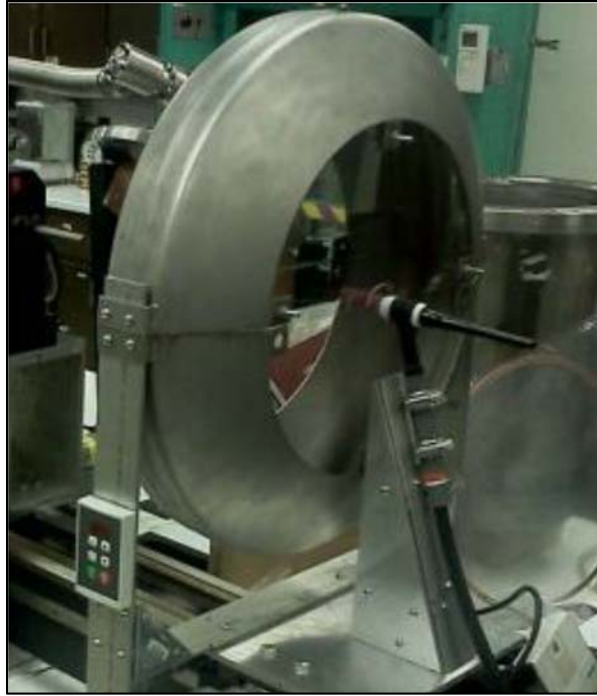
Figure 3-15: The catch pan without Plexiglas & aluminum inserts installed [1]
