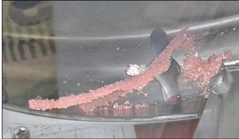
Figure 3-39: Conglomeration of copper microspheres
