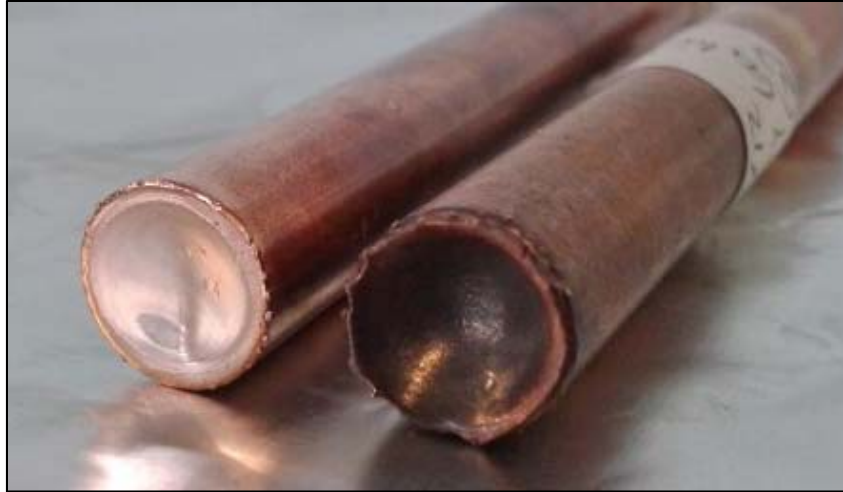
Figure 4-4: Contrast between copper rods melted in argon (left) and air (right) atmospheres
