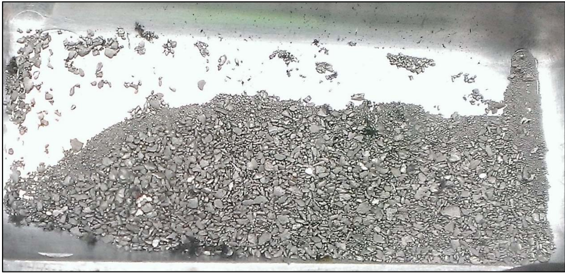
Figure 4-35: U-10Zr powder produced at 18,000 RPM using 50 A
