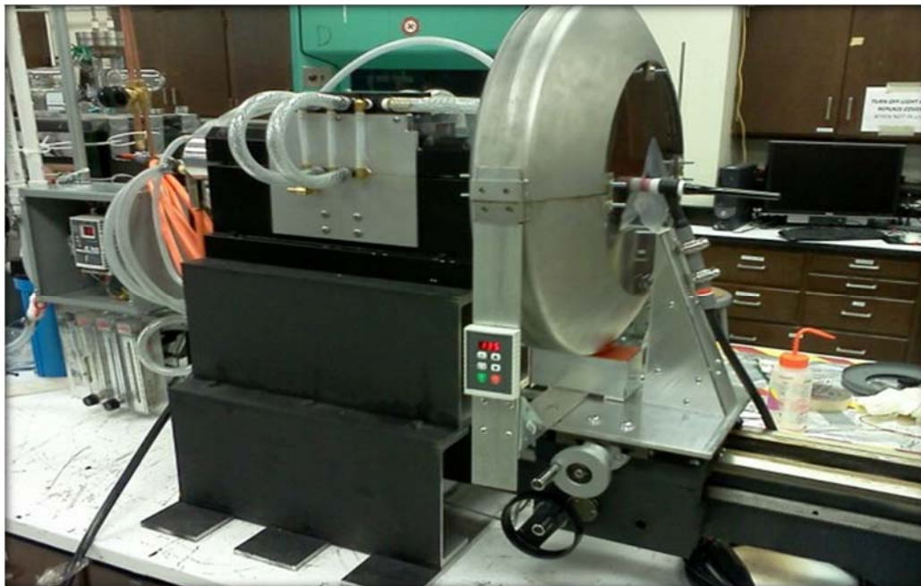
Figure 3-1: The Rotating Electrode System as built by Thompson [1]
