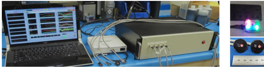
Fig. 73. The benchtop PPG sensor (on left) including the laptop, data acquisition card and sensor interface electronics (from left to right). The right panels show the visible (upper) and NIR LEDs (lower) used in this study.
