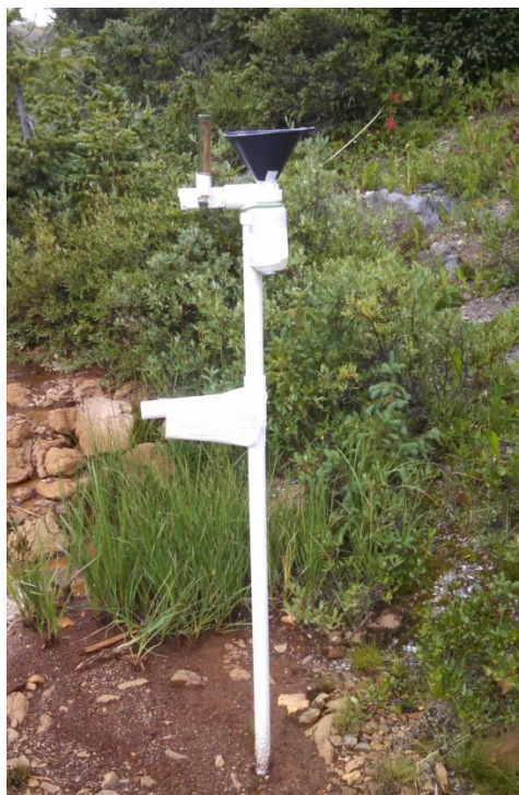
Figure 6. The deposition collector was constructed of PVC pipe with a funnel attached through the top of a 250 milliliter Nalgene sample bottle. A piece of 12.7 mm PVC was attached to the top of the collector to which a rain gauge was attached for precipitation quantification.
