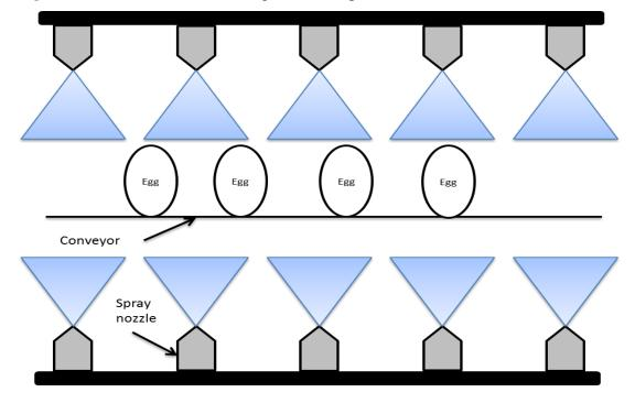
**Figure 6.** Third H<sub>2</sub>O<sub>2</sub> nozzle configuration (Experiment 7).
