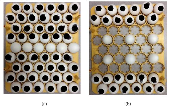
Based on the results from Experiment 6, it was determined that a further increase of  $H_2O_2$  spray was necessary to treat eggs on incubator flats. Therefore, a mist configuration that used 10 nozzles, 5 above of the conveyor and 5 below (Figure 7), was implemented for Experiment 7. In this experiment, eggs were treated on a full 168-egg plastic flat. Figure 8 illustrates the position of the 14 eggs sampled in this experiment. Additionally, 3 eggs were sampled as non-treated controls.
