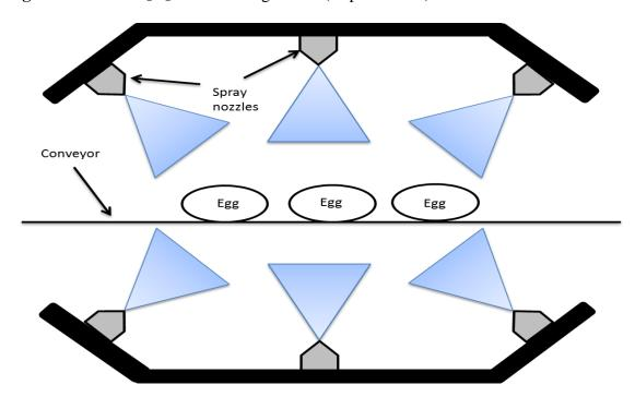
Figure 4. Second H<sub>2</sub>O<sub>2</sub> nozzle configuration (Experiment 6)
