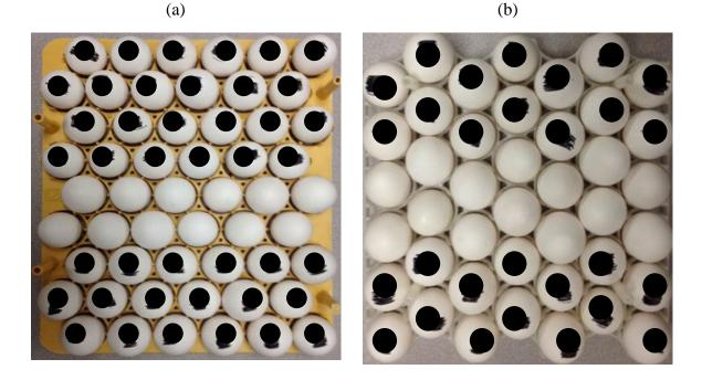
Based on the results from Experiment 5, it was hypothesized that an increased  $H_2O_2$  spray coverage was necessary to effectively treat eggs on commercial incubator flats. Therefore, 2 spray nozzles, 1 nozzle above the conveyor and 1 below it, were added to the original configuration (Figure 4). To further increase the egg exposure to  $H_2O_2$ , the conveyor was set to the 'slow speed' used in Experiment 2 (5.5 cm/s).
