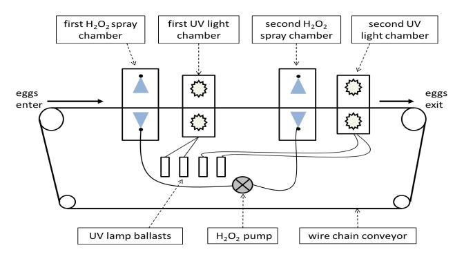
Figure 1. Schematic of  $H_2O_2/UV$  apparatus.
