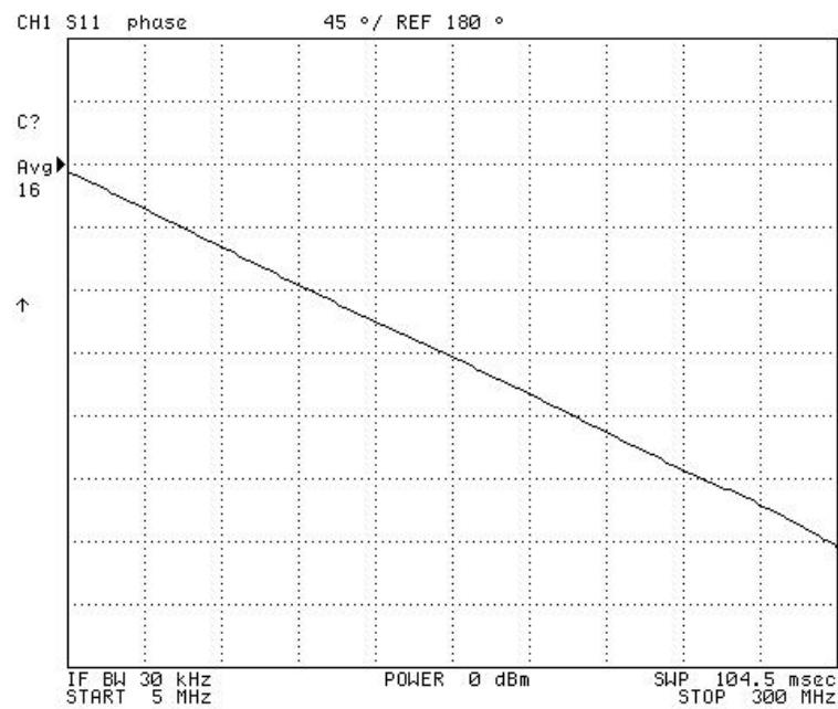
Figure II.29 Filter's phase response with a bandwidth of 150MHz
