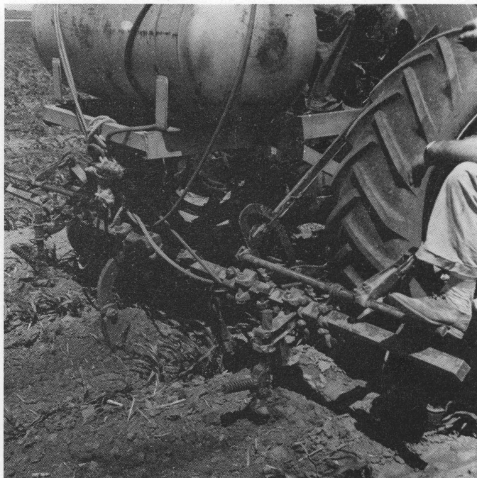
Fig. 4. Close-up of equipment for applying anhydrous ammonia. Nitrogen is released from under pressure in the tank, moves through the rubber hoses and is injected into the soil behind the knives.
