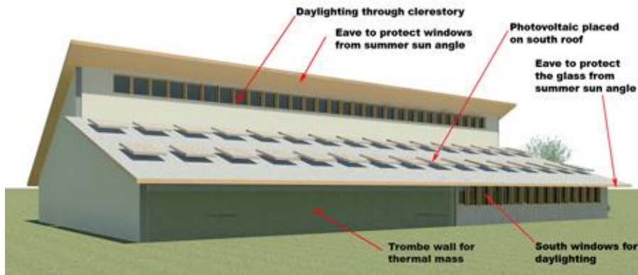
Figure 1. BIM model of the office building for solar simulations, Denver, 12 noon on August 25th 2010.
