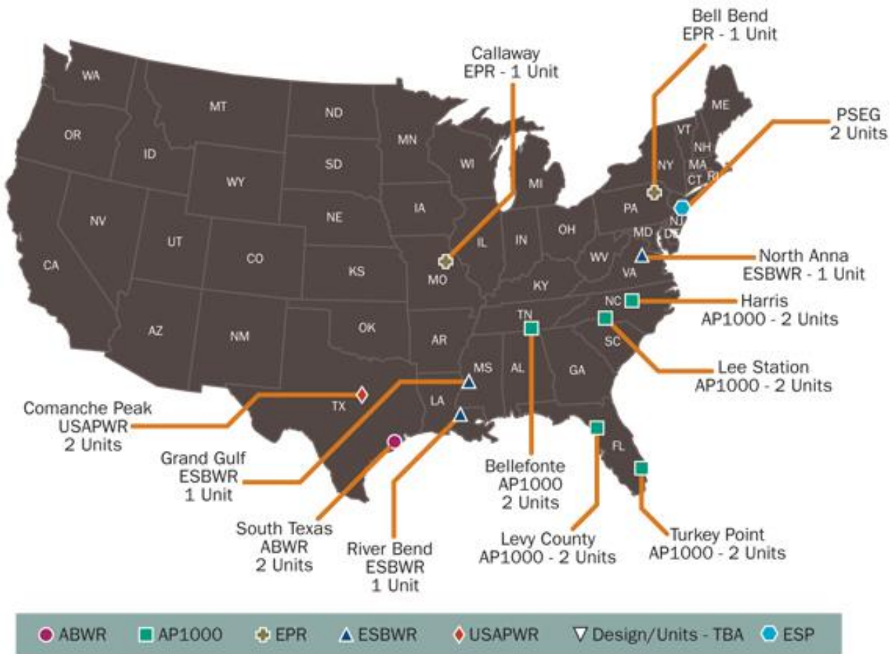
Fig. 10. Locations of projected new NPPs (ABWR: Advanced Boiling Water Reactor, AP1000: Advanced Passive 1000, EPR: Evolutionary Pressurized Reactor, ESBWR: Economic Simplified Boiling Water Reactor, USAPWR: US Advanced Pressurized Water Reactor, ESP: Early Site Permit) (USNRC 2015d).
