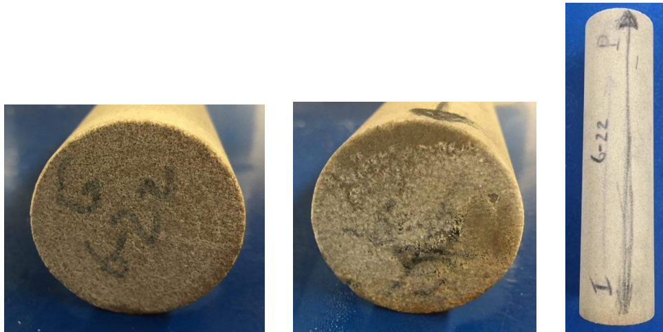
Fig. 15—Injection Face, Production Face, and Side View of Berea-G-6-22 After Acid Treatment.
