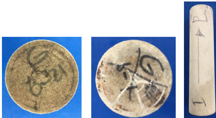
Fig. 78—Injection Face, Production Face, and Side View of Berea-G-6-21 After Acid Treatment.
