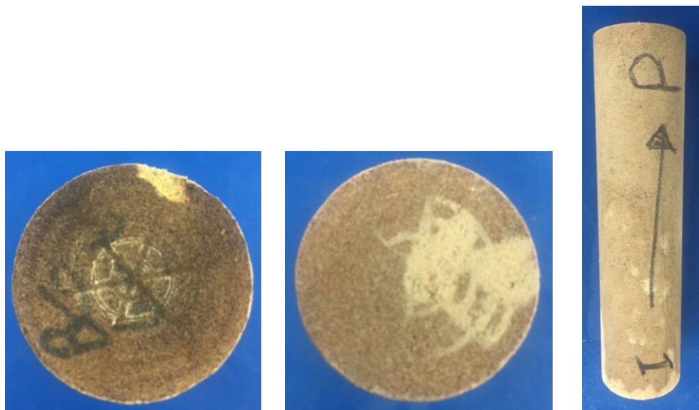
Fig. 48—Injection Face, Production Face, and Side View of Bandera-BG-6-6 After Acid Treatment.
