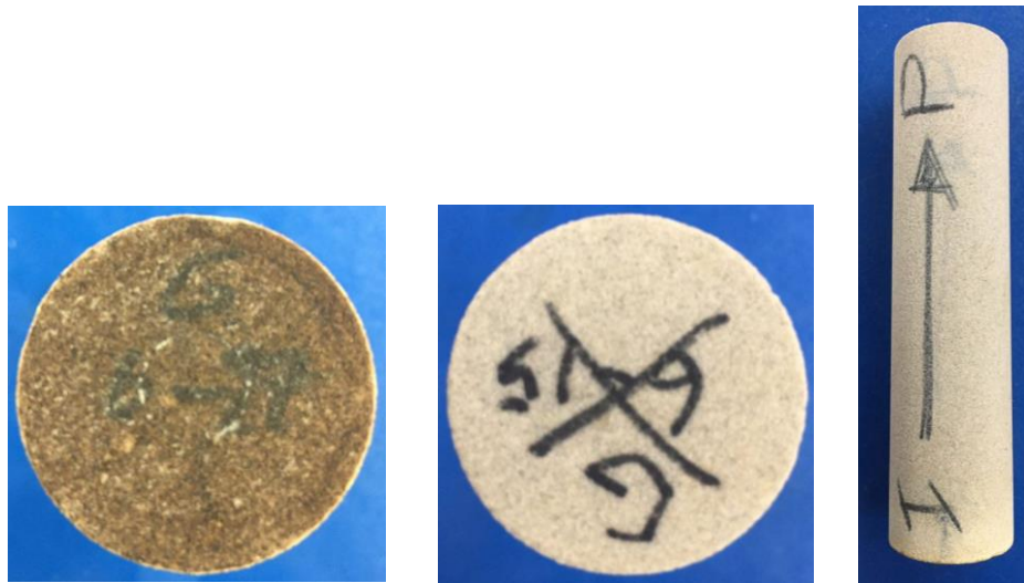
Fig. 41—Injection Face, Production Face, and Side View of Berea-G-6-27 After Acid Treatment.
