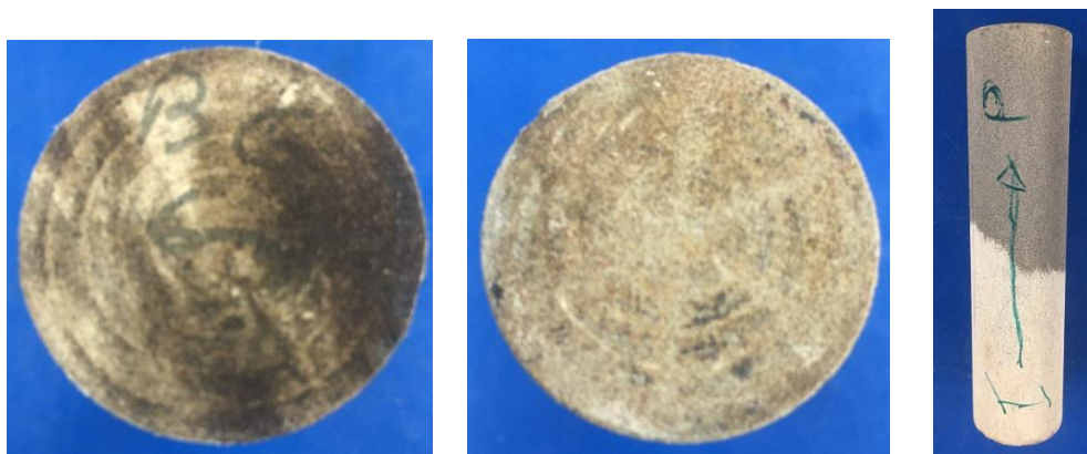
Fig. 85—Injection Face, Production Face, and Side View of Bandera-BG-6-7 After Acid Treatment.
