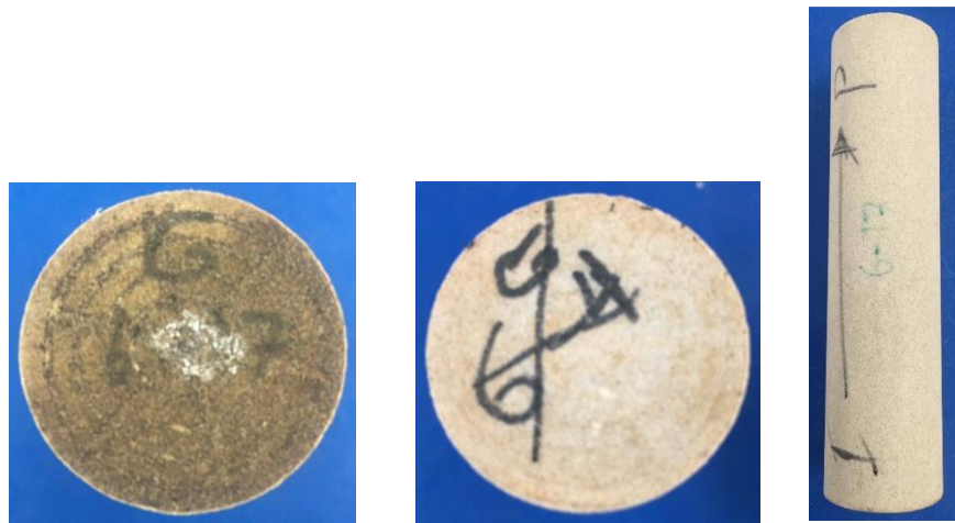
Fig. 101—Injection Face, Production Face, and Side View of Berea-G-6-17 After Acid Treatment.
