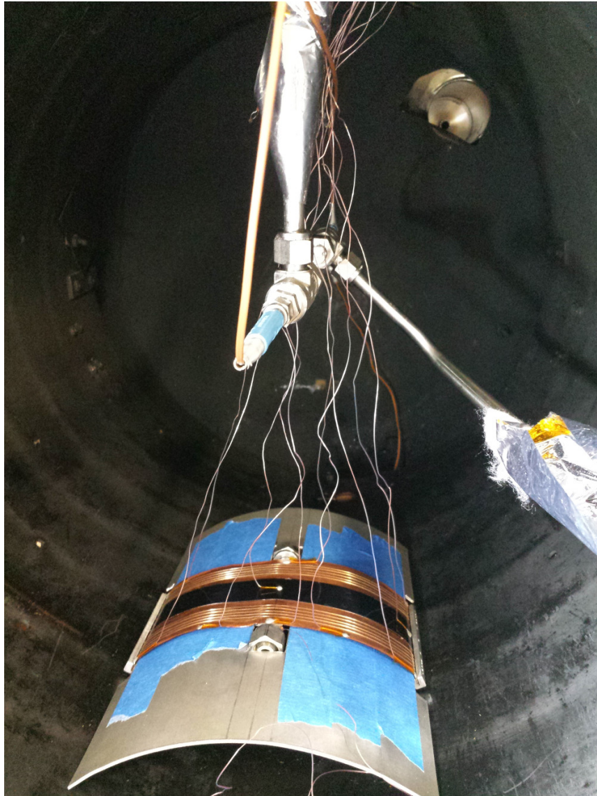
Figure 4.9: Photograph showing morphing radiator on the assembly jig just prior to being installed in the vacuum chamber.
