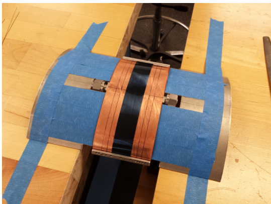
(e) After attaching spring steel strip.
