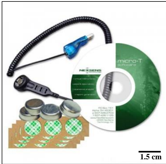
Figure 2.7. Three NexSens DS1923 Micro-T temperatures loggers randomly placed on the anti-scavenging cages (approximately 0.3 m above the ground) in the field located at Snook, Texas during summers 2013 and 2014. (Image downloaded from http://www.fondriest.com/reviews/humidity-sensors ) (Accessed on 22 March 2015).
