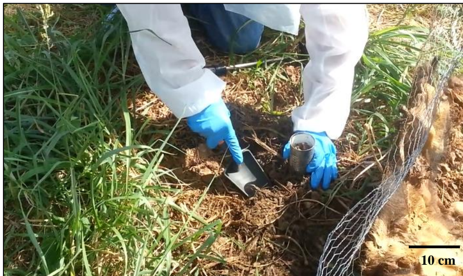
Figure 2.13. Collection of soil beneath the pig, Sus scrofa L., carcass using a sanitized plastic trowel. The soil was then transferred into a sterilized tin can (170 g capacity), and poured into a Ziploc bag, and mixed. The soil samples were then kept in a cooler at 4°C and transported to lab.
