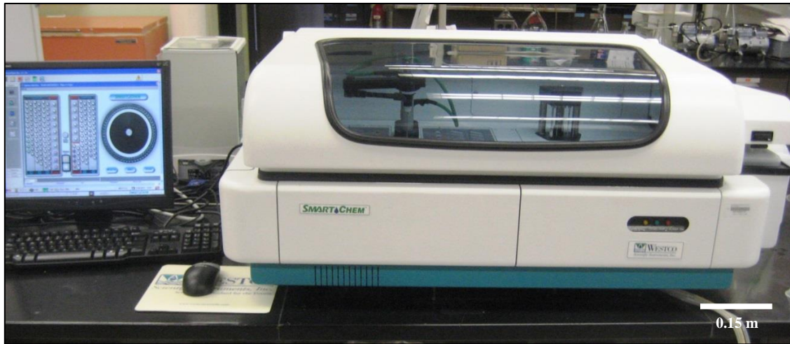
Figure 3.3. SmartChem Discrete Analyzer (located at the NAWA lab, Texas A&M University) used to measure soil nutrient concentrations ( \text{NO}_3\text{-N} , \text{NH}_4\text{-N} and \text{PO}_4\text{-P} ) from the soil samples collected in both summers 2013 and 2014 at the field site located at Snook, Texas.
