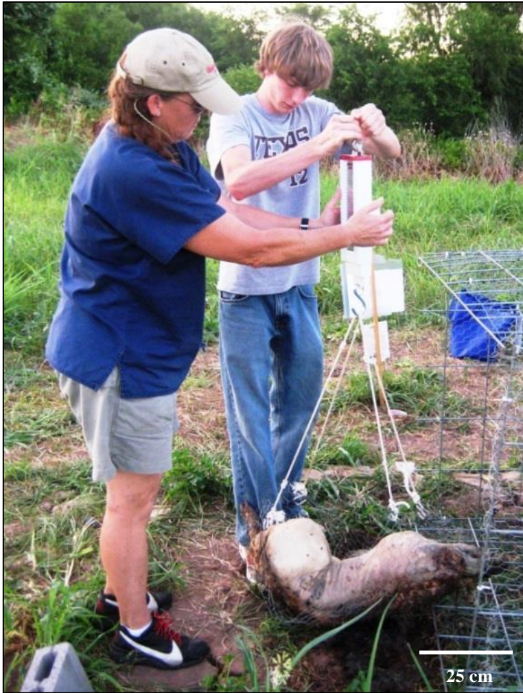
Figure 2.9. Weighing of pig, Sus scrofa L., carcass biomass in the field using a hanging scale during summers 2013 and 2014 at Snook, Texas. A sterilized platform made of aluminium mesh (0.9 m x 1.2 m) was placed at the bottom of each swine carcass for lifting purposes.
