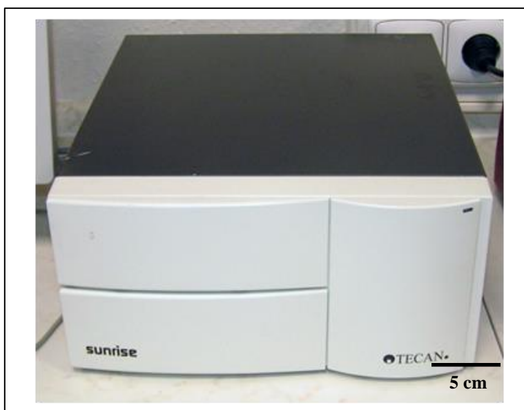
Figure 2.15. Plate reader Tecan Sunrise™ used in this study to measure average OD of Biolog EcoPlate™ for both 2013 and 2014 trials (Image downloaded from http://www.biotrans.cas.cz ).
