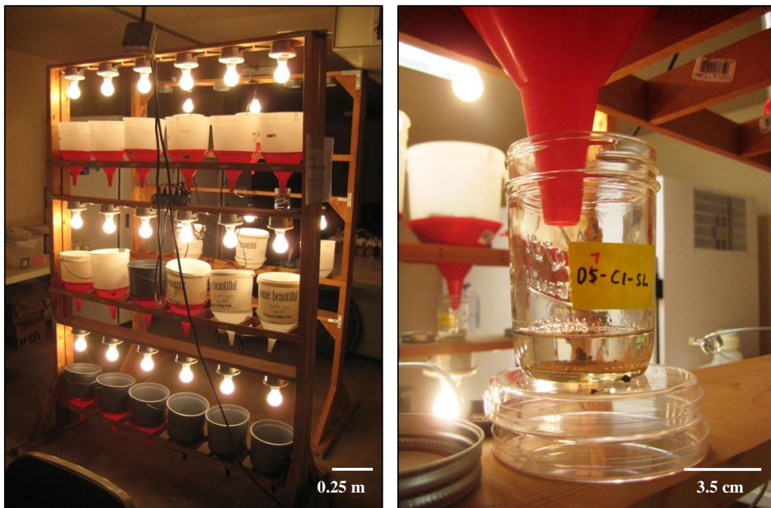
Figure 4.1. Left. Berlese funnels and the racks used to extract soil arthropods from soil samples collected from the field site at Snook, Texas during summers 2013 and 2014. Right. Mason jar containing 70% ethanol to preserve extracted soil arthropods from Berlese funnels.
