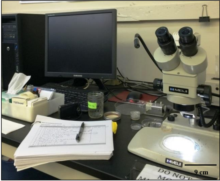
Figure 4.3. The stereo microscope (Meiji, Japan) used in sorting and identifying soil arthropods collected from the field site at Snook, Texas in summers 2013 and 2014.
