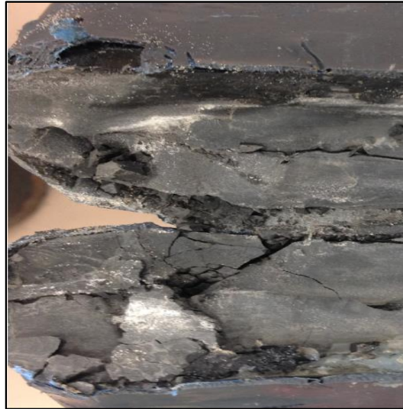
Fig. 2.22 – Damaged Sample from Facies B After 100 Mesh Experiment.
