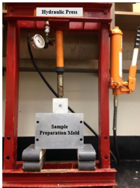
Fig. 2.25 – Removing the Conductivity Sample Coated With Epoxy from the Sample Preparation Mold.
