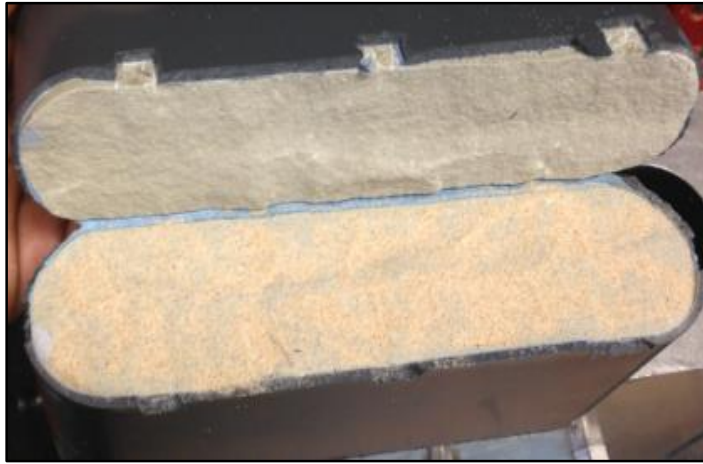
Fig. 2.28 – Conductivity Sample with 0.1 lbm/ft 2 - 100 Mesh.
