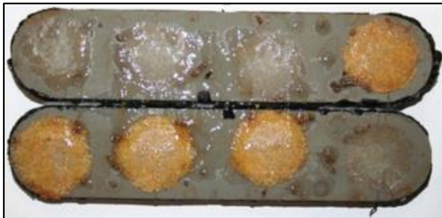
Fig. 1.3 –Proppant Arrangement with Proppant Pillars and Channels on a Fracture Conductivity Sample (Gillard et al. 2010).
